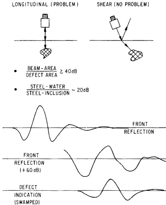
Figure 1. Near surface inspection.
