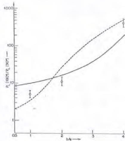
Figure 2. The ratio  $P(180)/P(90)$  for longitudinal power with longitudinal wave incident along symmetry axis of spheroidal cavities in Ti, vs.  $b/a$  of the scatterer. Uniform averages of  $0 < ka < 1$  (full lines) and  $9 < ka < 2$  (broken lines) were used. The circles are experimental results.
