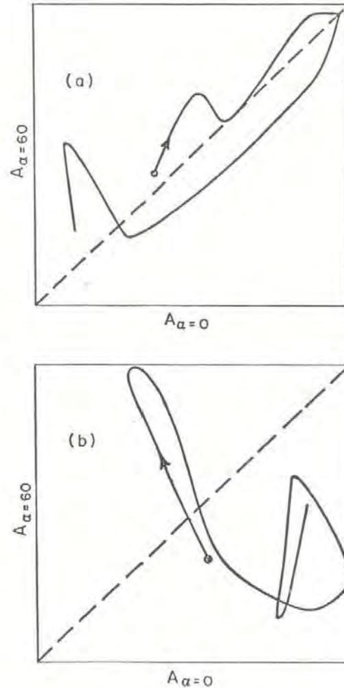
Figure 9. Plot of equally normalized amplitude,  $A_{60}(f)$  vs.  $A_0(f)$ , using the frequency  $f$  as a parameter. The heavy dot indicates  $f = 2$  MHz, and the arrow the direction of increasing  $f$ . The dashed line is the expected curve for a spherical defect.
