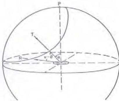
Figure 7. Geometry of experimental setup used to determine line of symmetry. The transmitter, T, is at the center of the window;  $\alpha$  is the angle between the direction of incidence and the symmetry axis of the defect. This axis intersects the window at P. R is position of receiver,  $\theta$  is the scattering angle. To determine the orientation we want to locate P. The line of symmetry connects P and T.
