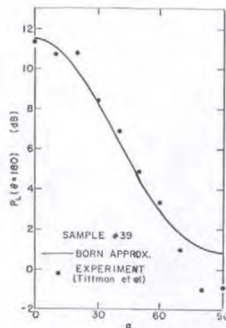
Figure 3. Backscattered longitudinal power  $P_L(\theta=180^\circ)$ , as a function of angle of incidence,  $\alpha$ , for spheroidal cavity ( $b=400\mu$ ,  $a=200\mu$ ) in titanium. Rockwell transducer characteristics were used for the frequency averaging. The line is the Born approximation; dots are measurements (Tittmann, et al.).
