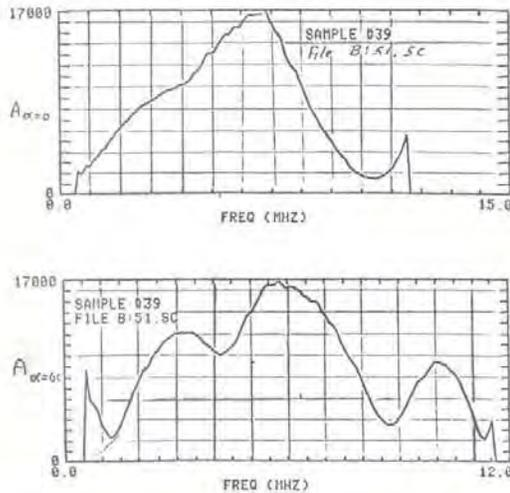
Figure 8. Amplitude vs. frequency of backscattered wave from oblate spheroid ( $b = 400\mu$ ,  $a = 200\mu$ ) in Ti, for angle of incidence  $\alpha = 0^\circ$ , and  $\alpha = 60^\circ$ .
