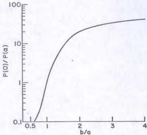
Figure 4. Ratio of backscattered power at  $\alpha = 0$  and  $\alpha = 90^\circ$ , vs.  $b/a$ , for spheroidal cavities in titanium: Born approximation.
