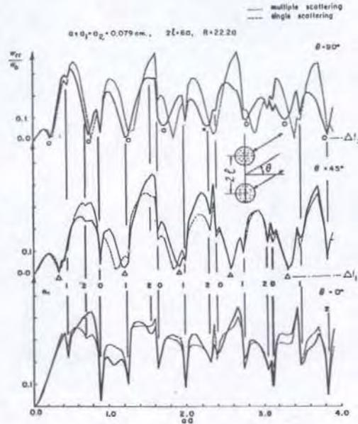
Figure 10. Backscattering of P-waves by two circular water cylinders at various angles of incidence ( $\sigma_{rr}$  is the radial stress,  $\omega a = \omega a / c_p$ )<sup>13</sup>.
