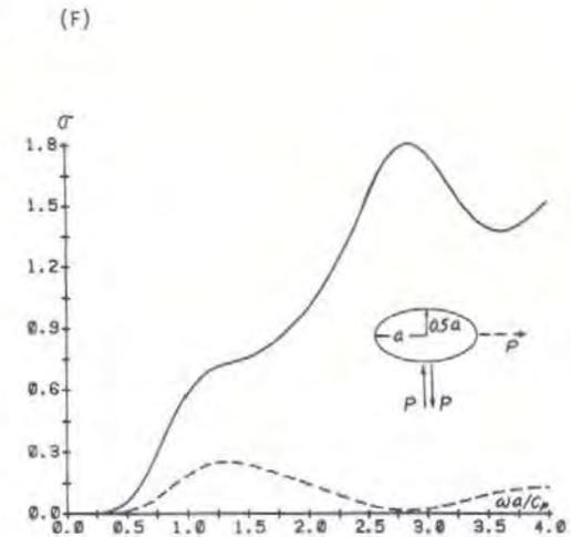
Figure 7. Backscattering and right-angle scattering of P-waves by an oblate spheroid ( $\sigma$  is the differential cross section).
