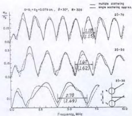
Figure 9. Backscattering of P-waves by two circular cylindrical cavities separated by a distance  $2b$ , incident at an angle  $\theta = 30^\circ$  with the horizontal axis ( $\sigma_{rr}$  is the radial stress at distance  $R = 32a$  from the mid-point of two circles)<sup>13</sup>.
