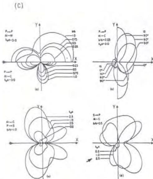
Figure 4. Angular distribution of far field scattered wave amplitudes by an elliptical cylinder with major axis  $2a$  (along x-axis) and minor axis  $2b$ . (Al-W indicates tungsten cylinder in aluminum matrix; Al-C indicates a cavity in aluminum solid;  $\alpha$  the incident angle with respect to the x-axis).
