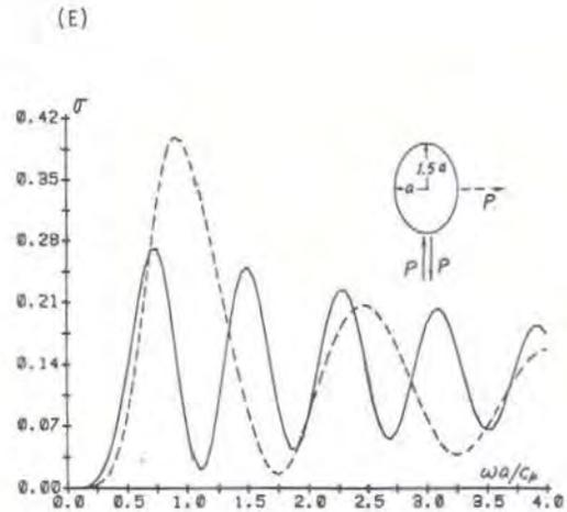
Figure 6. Backscattering and right-angle scattering of P-waves by a prolate spheroid ( $\sigma$  is the differential cross section).
