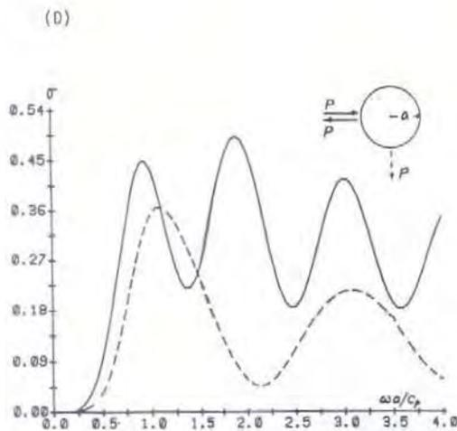
Figure 5. Backscattering and right-angle scattering of P-waves by a spherical cavity of radius 'a' ( $\sigma$  is the differential cross section).
