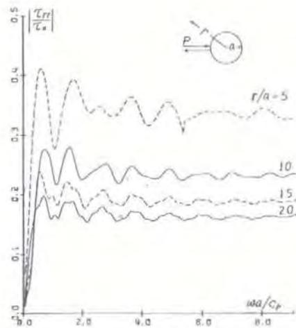
Figure 2. Backscattering of P-waves (longitudinal waves) by a circular cylindrical cavity ( $T_{rr}$  is the radial stress,  $c_p$  the P-wave speed in solid).
