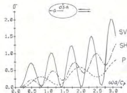
Figure 3. Backscattering by an elliptic cylindrical cavity for an incident P, SV (transversely polarized shear) and SH (horizontally polarized shear) wave along the major axis ( $a$  is the differential cross section).
