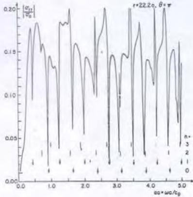
Figure 8. Backscattering of P-waves by a circular cylindrical cavity filled with water ( $\sigma_{rr}$  is the radial stress at distance  $r = 22.2a$ ).
