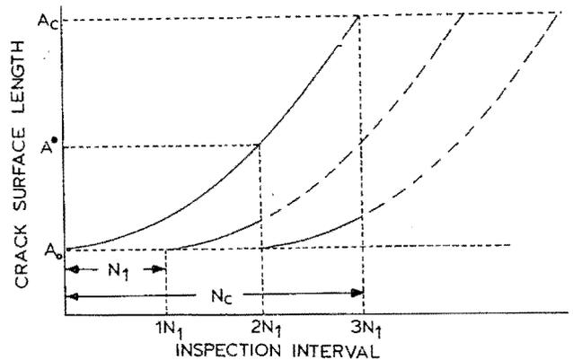
Fig. 1. Crack growth - NDE relationship for Retirement for Cause program.
