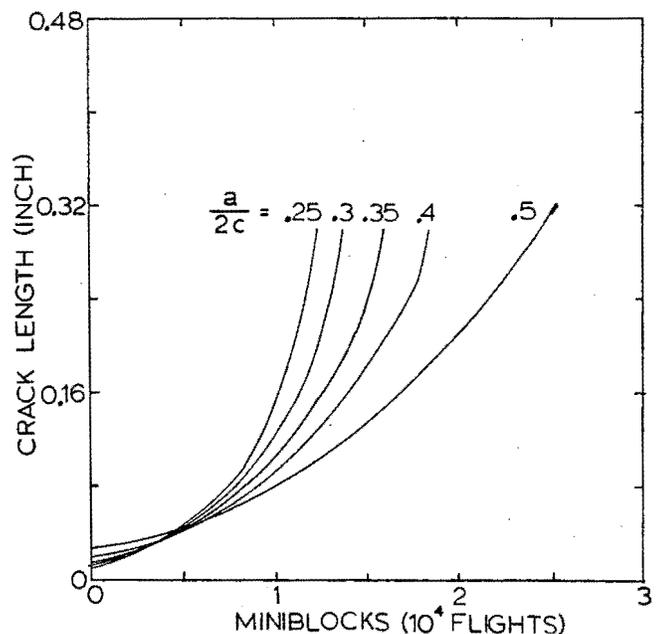
Fig. 2. Crack growth as a function of aspect ratio for 3rd stage turbine disk in the TF-33 engine.
