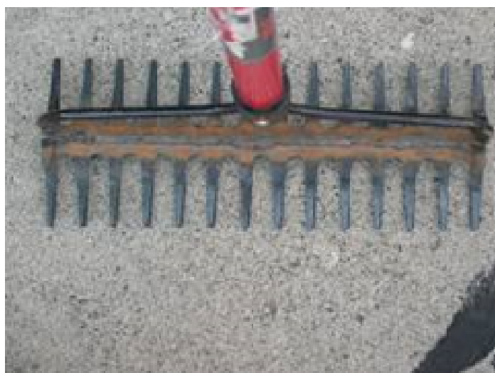
FIGURE 1. Double sided rake as described in Yin et al. (2000) used to collect macrophytes samples (Clayton et al. 2007).
