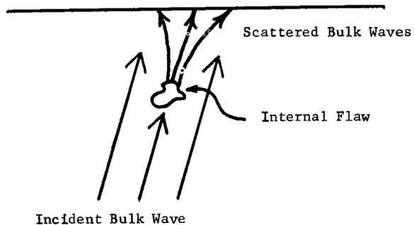
Fig. 12 - Insonification of sample having a void or inclusion deep beneath the surface.
