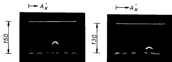
Fig. 8 Compound scan imaging of a cylindrical side drilled hole and a bottom hole with  $32^\circ$  cone.
