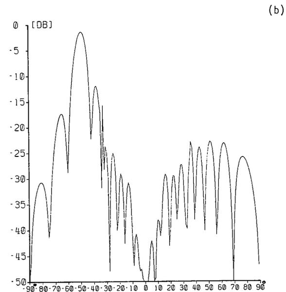
Fig. 2 Directivity pattern of a steered  $50^\circ$ , 20 element array with shear wave excitation. (a) 500 Hz clock frequency; (b) 10 kHz clock frequency.
