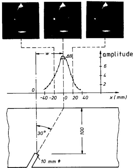
Fig. 6 Sector display and compound-scan-amplitude-locus curve of a planar defect.
