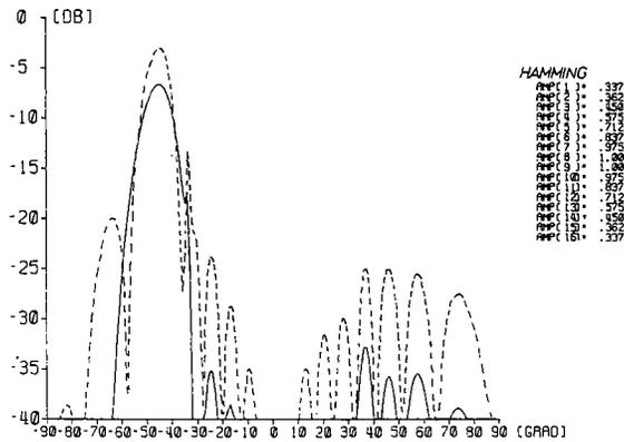
Fig. 3 Array-Shear-Wave-Beam-Pattern, 45° steered, with and without Hamming-weighting.
