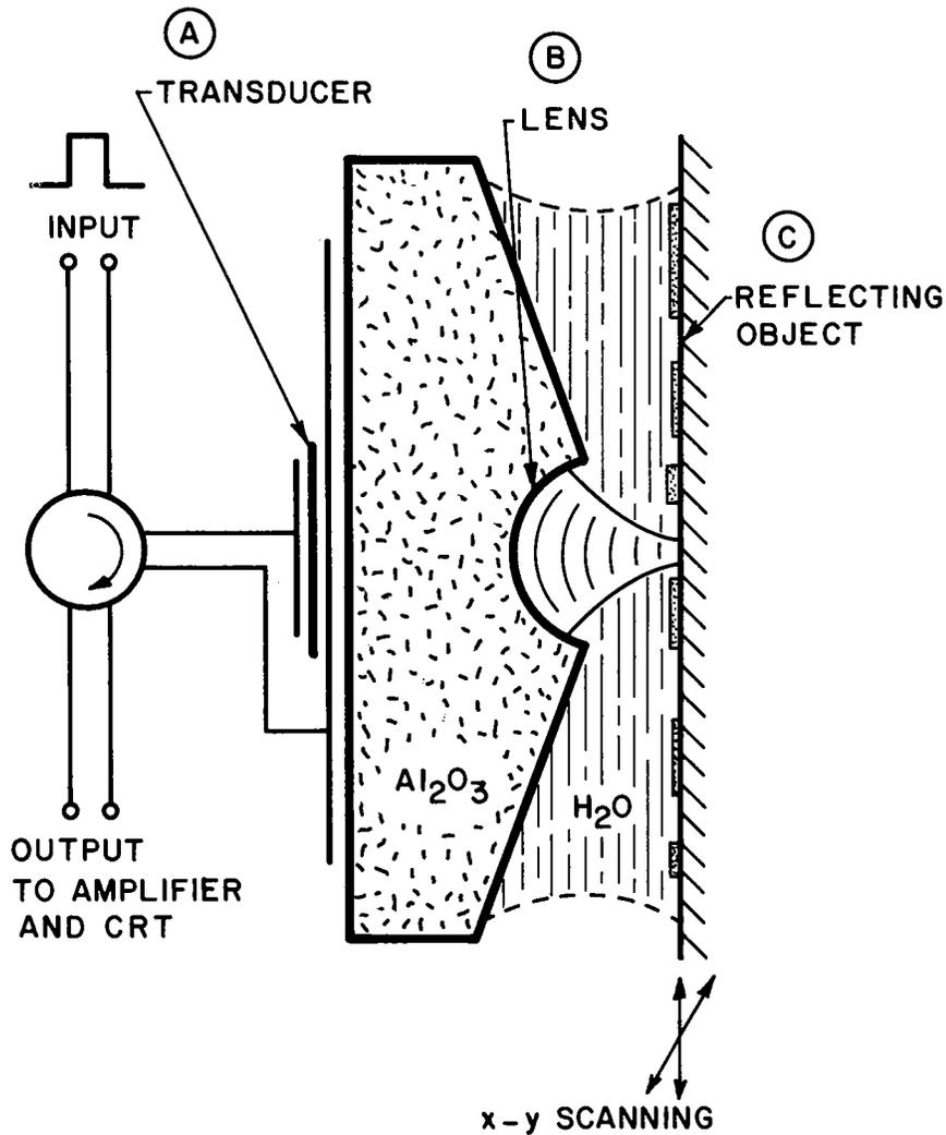
FIG. 1--Acoustic lens.
