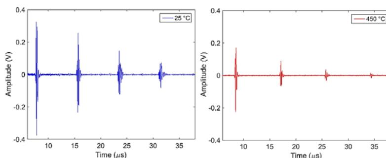
**Figure 1.** Ultrasonic A-scans with four consecutive back-wall echoes on a magnetite coated 12 mm thick steel sample at 25 °C (left) and 450 °C (right) with 512 averages
