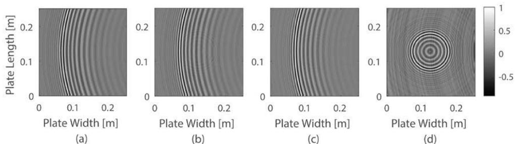
**Figure 1.** Wavefield snapshots. (a) Baseline measurement without damage. (b) Current measurement with damage and a 1% velocity change. (c) Direct difference of (a) and (b). (d) Difference using fitted baseline data.
