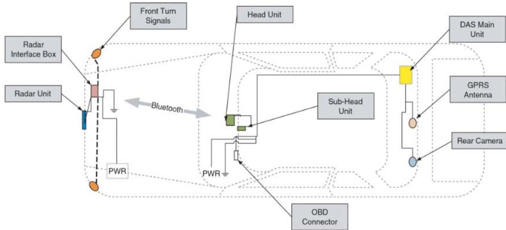
**Figure 4.** Data acquisition system schematic (Antin et al., 2011)
