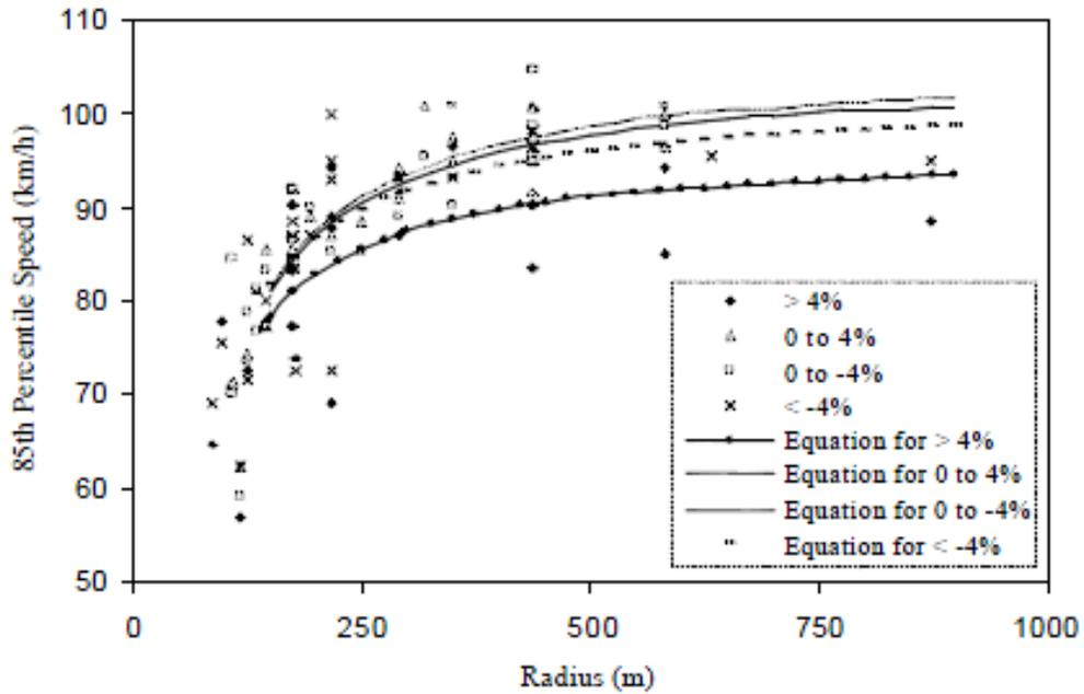
**Figure 3.** 85<sup>th</sup> percentile speed versus radius along horizontal curves on grades (FHWA, 2000)
