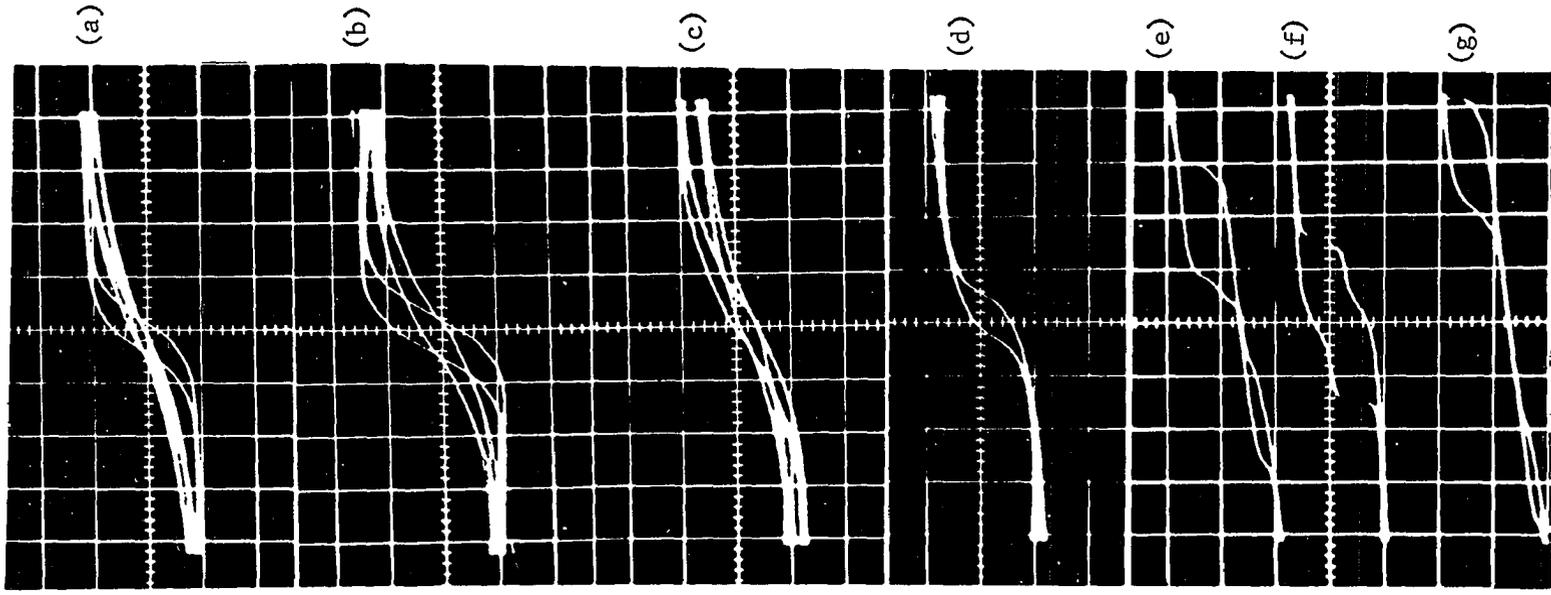
required in the operation of the thin film parametric amplifier at the low temperature than at room temperature. The increased loss as evidenced by the opening of the 60 cps hysteresis loop was obviously due to domain rearrangement and consequently would add greatly to the Barkhausen noise.
