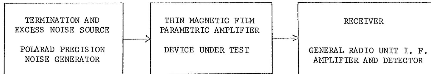
Figure 10. The system and equipments used for noise measurement
