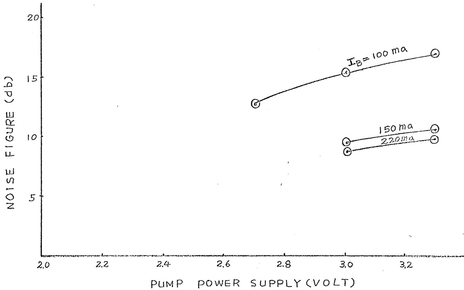
Figure 15. Measured noise figures of thin film parametric amplifier using thin film inductor B when film is cooled to about liquid nitrogen temperature
