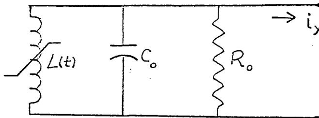
Figure 3. Idealized equivalent circuit of the thin film inductor
