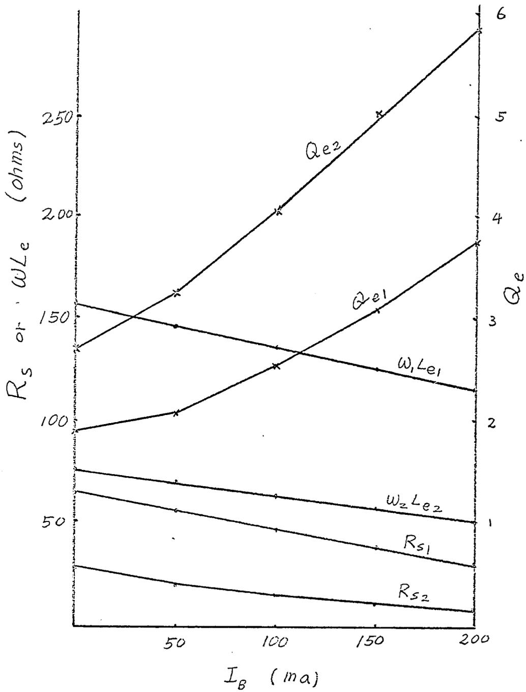
Figure 8. The static characteristics of the thin film inductor C. The subscripts 1 and 2 refer to the values at 30 mc/s and 15 mc/s respectively
