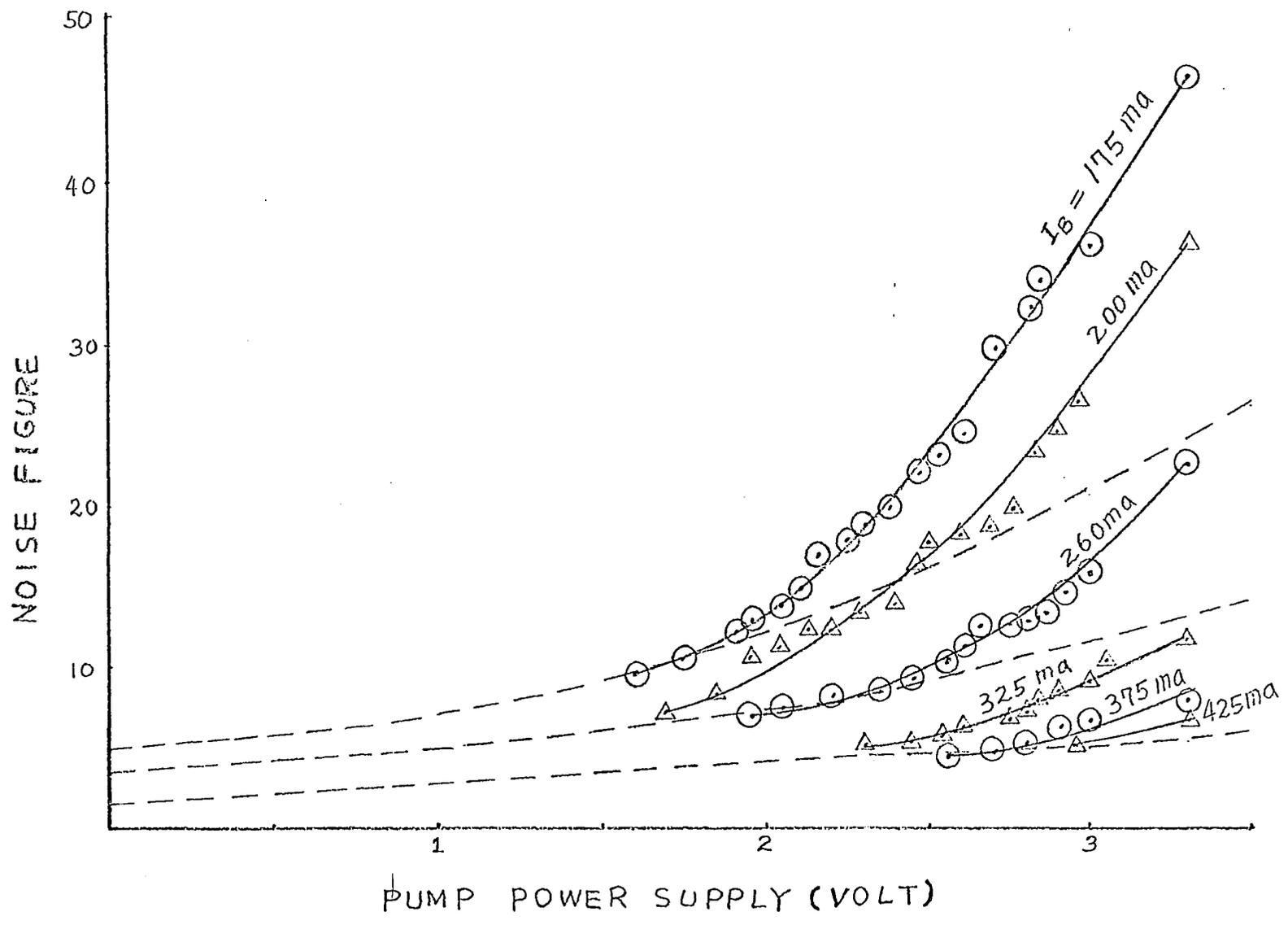
Figure 19. Measured noise figures of the thin film parametric amplifier using thin film inductor B but with a different film at room temperature
