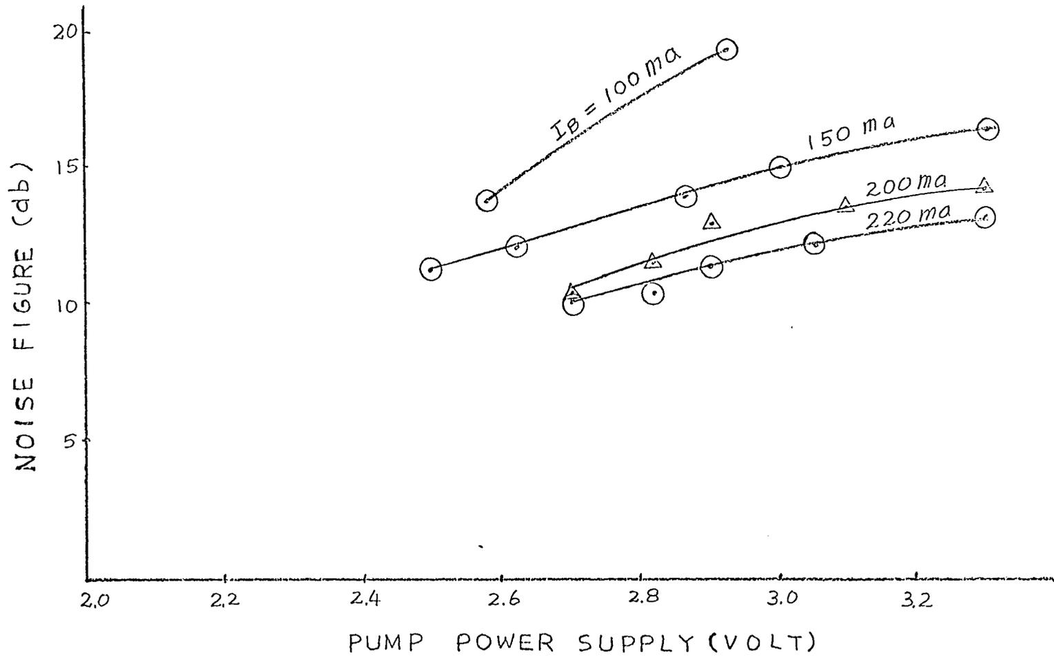
Figure 16. Measured noise figures of the thin film parametric amplifier using thin film inductor C with respect to different bias current at room temperature
