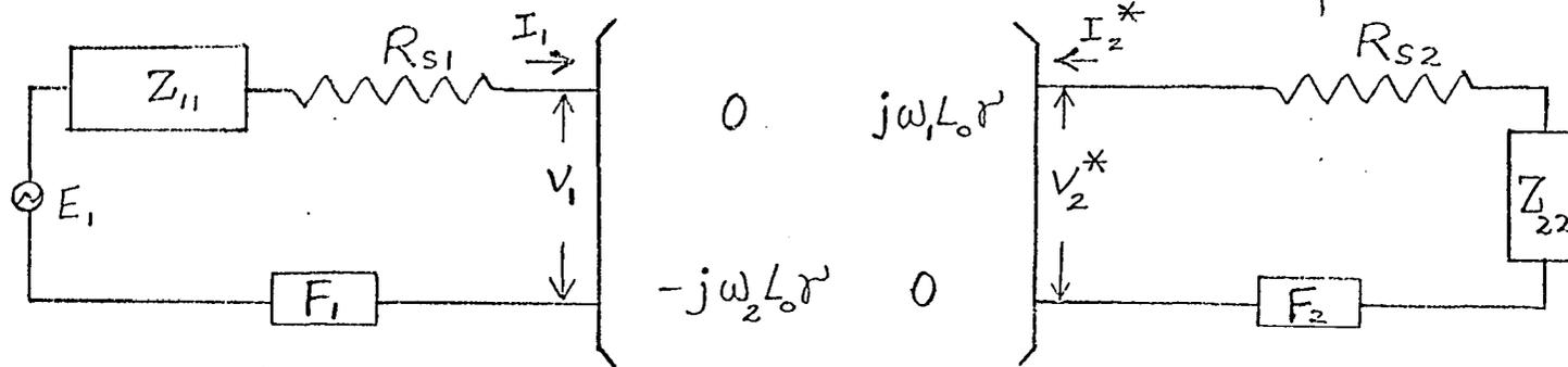
Figure 4. The circuit model for inverting type parametric devices.  $F_1$  and  $F_2$  are bandpass filter
