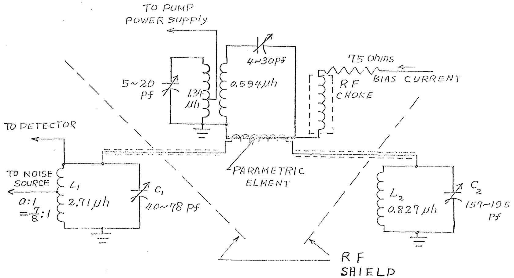
Figure 9. The schematic diagram of the thin magnetic film parametric amplifier for noise measurement
