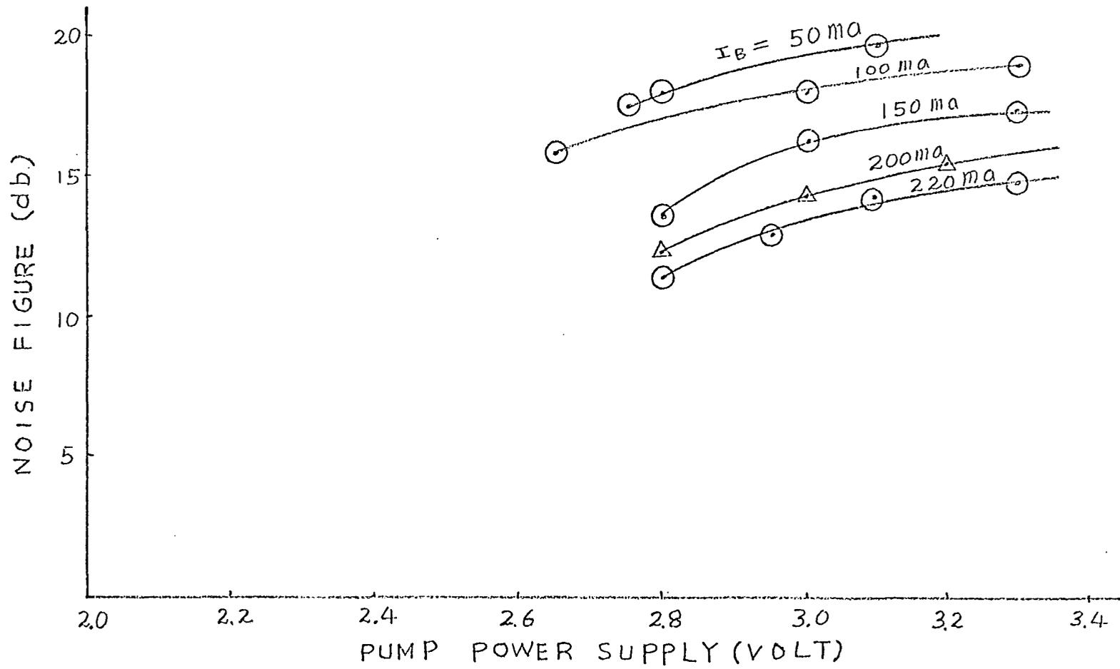
Figure 18. Measured noise figures of the thin film parametric amplifier using thin film inductor B with different bias currents at room temperature. Abscissa is calibrated to 274 ma (rms)/volts
