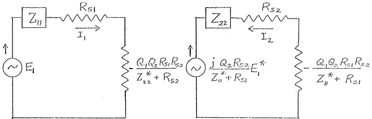
Figure 5. The linearized equivalent circuits for signal and idler circuits
