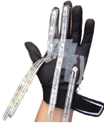
Figure 3: Force sensors on hand during Catching Test
