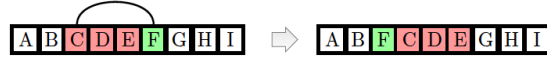
Figure 2.6: Example of the insertion operator. The variable F is inserted at the position of variable C in the initial ordering
