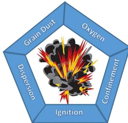
**Figure 1. Grain dust explosion pentagon. Reproduced from “Agricultural Dust Explosions” by Ambrose, R.P.K., 2017. Internal document from Purdue University.**
