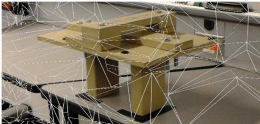
Figure 3.3. HoloLens' spatial mapping of a basic assembly.
