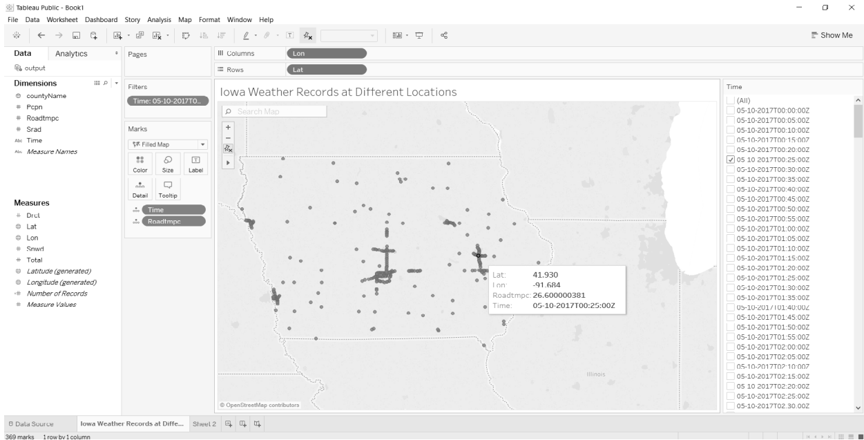
Figure 4.8 This Tableau dashboard shows the road temperatures in degree Celsius at different times of the day at different locations. We can select the time from the time selector panel on the right. And once hovering the marker we'll be able to see the road temperature at that location at that time.
