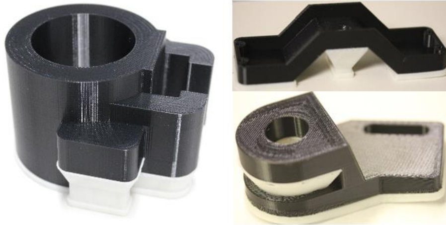
Figure 1 Removal of support structures in FDM may damage printed parts and generate chemical hazards
