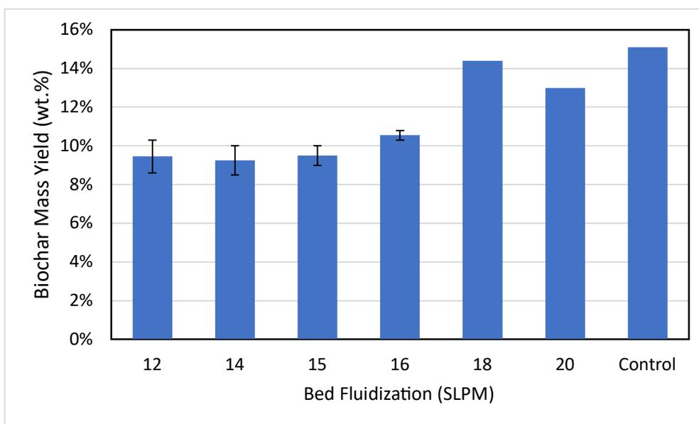
Figure 4.9 Mass yield of biochar throughout different in-bed injection tests. Control was performed at 20 SLPM with in-bed injection.
