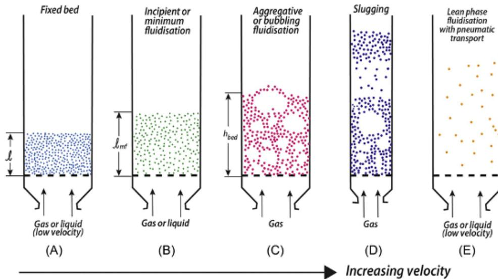
Figure 2.1 Representation of a fluidized bed as superficial velocity increases. (a) the starting bed height; (b) minimum fluidization with a bed height of ( $l_{mf}$ ) as fluidization begins; (c) corresponds to a fluidized bed with properly sized bubbles; (d) slugging regime occurs with large bubble formation; (e) is an entrainment bed in which particles are mostly all removed [16].
