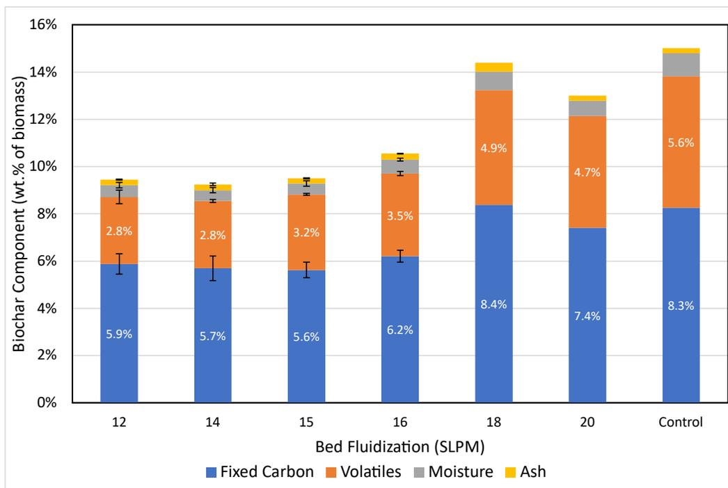
Figure 4.8 Impact of bed fluidization on the amount of biochar components present. Control test is at 20 SLPM in-bed injection.
