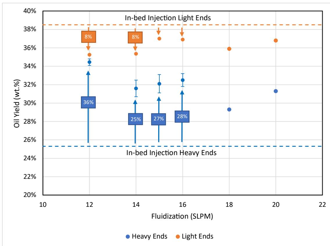
Figure 4.4 Heavy and light end yields for red oak above-bed injection at different fluidization velocities (error for light ends was less than 0.5 wt.%). The dashed lines represent the in-bed control test with red oak at 20 SLPM.
