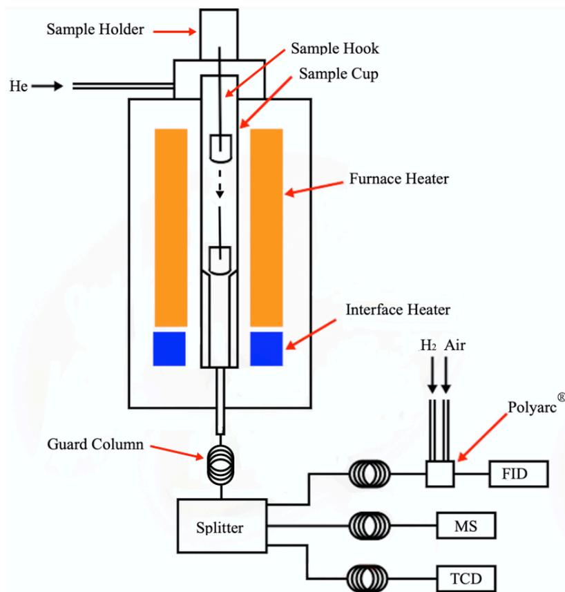
Figure 3.2 Schematic of micropyrolyzer with GC analysis of products. Pyrolysis vapors released from the sample in the furnace are swept into one of three GC columns for identification via MS or quantification via Polyarc/FID or TCD.
