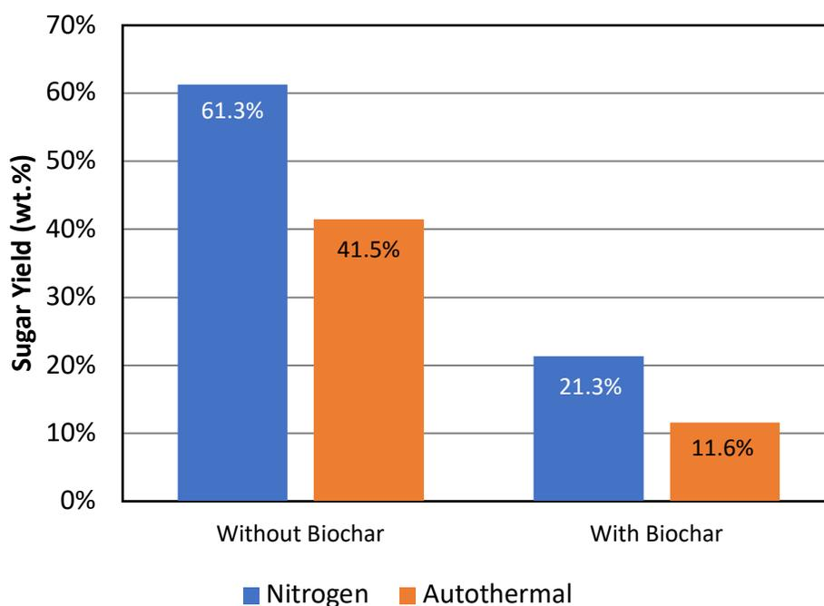
Figure 4.3 Result of adding untreated corn stover biochar to cellulose while running a fluidized bed reactor in both autothermal and conventional pyrolysis conditions. Autothermal runs maintained an equivalence ratio of 12% throughout testing, but temperatures were unable to stay steady without the added biochar
