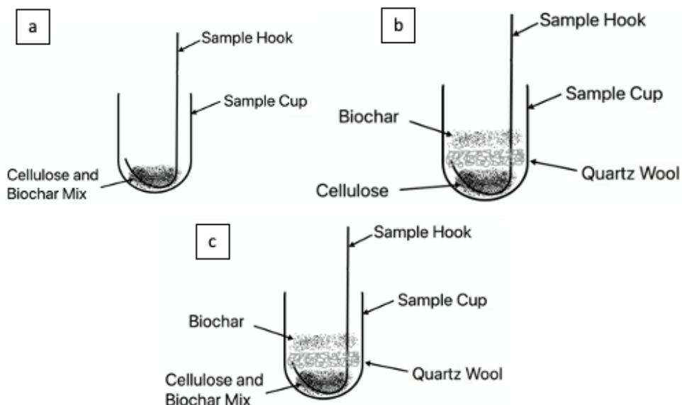
Figure 3.1 Biochar loading into the sample cup during micropyrolysis experimentation. Figure (a) showcases only the cellulose and biochar mixture; (b) demonstrates pure cellulose with a biochar layer; (c) has both a cellulose/biochar mixture and a layer of biochar
