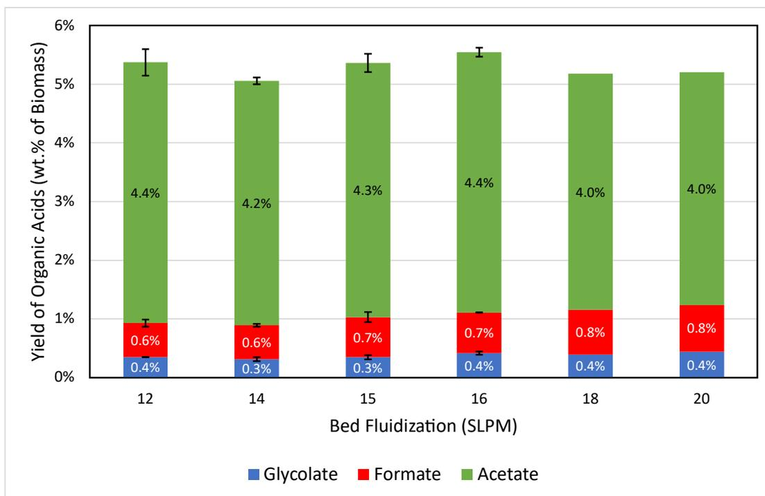
Figure 4.6 Effect of different fluidization rates on the decomposition of products to acids.
