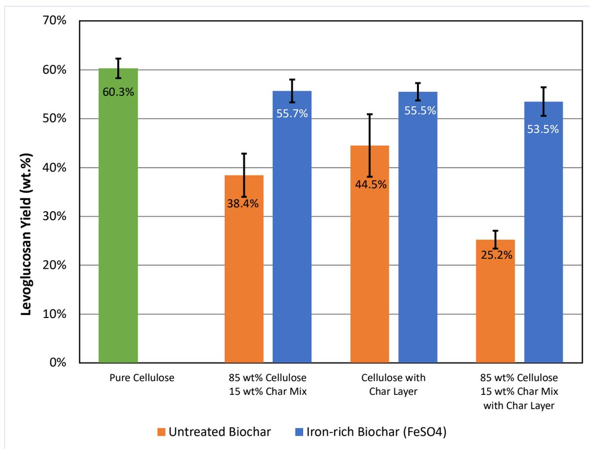
Figure 4.1 Untreated biochar reduced yields of levoglucosan while pretreated biochar did not substantially degrade levoglucosan yields.
