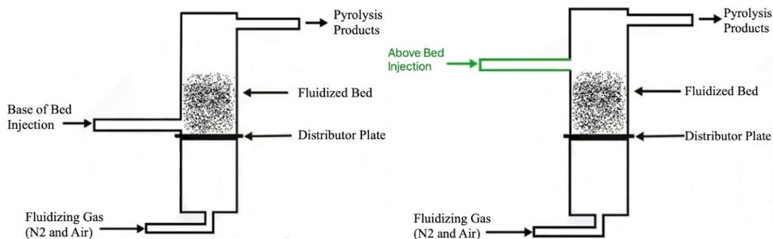
Figure 3.3 Diagram showing a cross section view of change being made which shows the base of bed injection (left) versus the new above bed injection (right).
