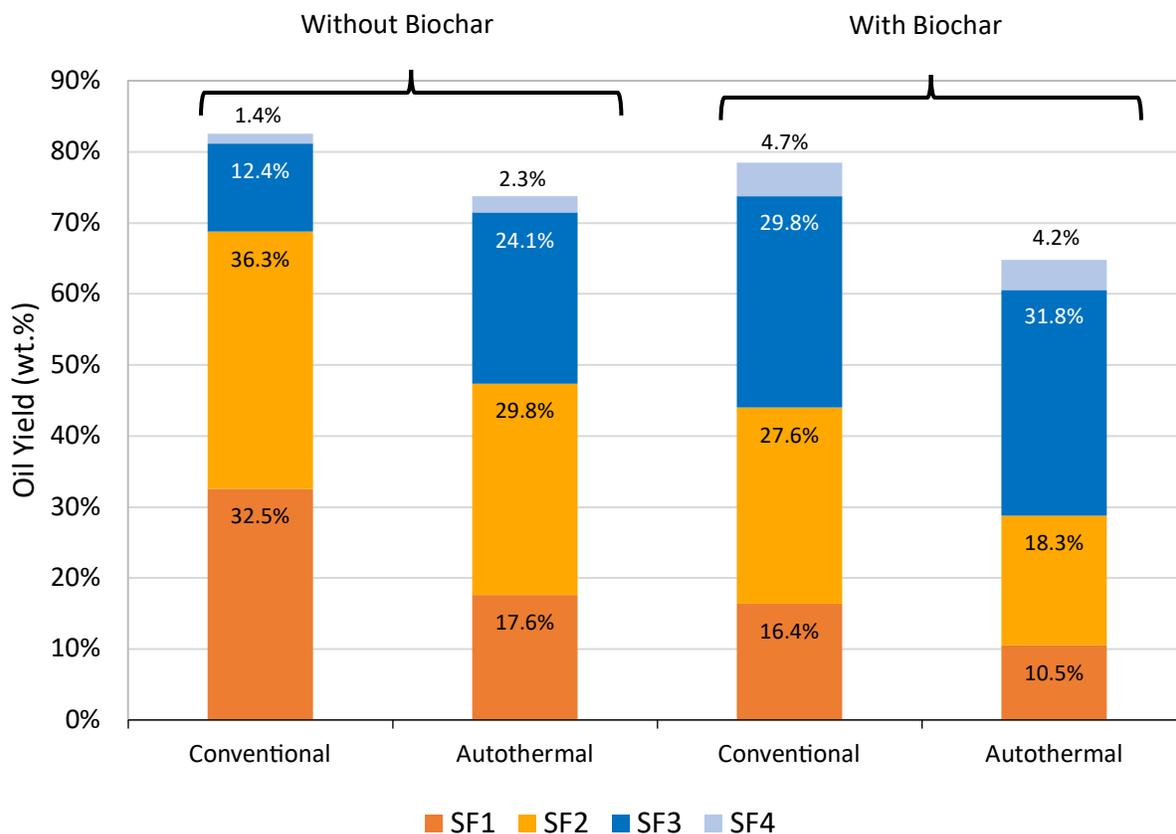
Figure 4.2 Yield of heavy ends (SF1 and 2) and light ends (SF3 and 4) from pyrolysis of cellulose in a continuous fluidized bed reactor under conventional ( $N_2$ ) and autothermal (AT) conditions. The tests with biochar consist of 85 wt.% cellulose 15 wt.% untreated corn stover biochar, while the other tests are pure cellulose.
