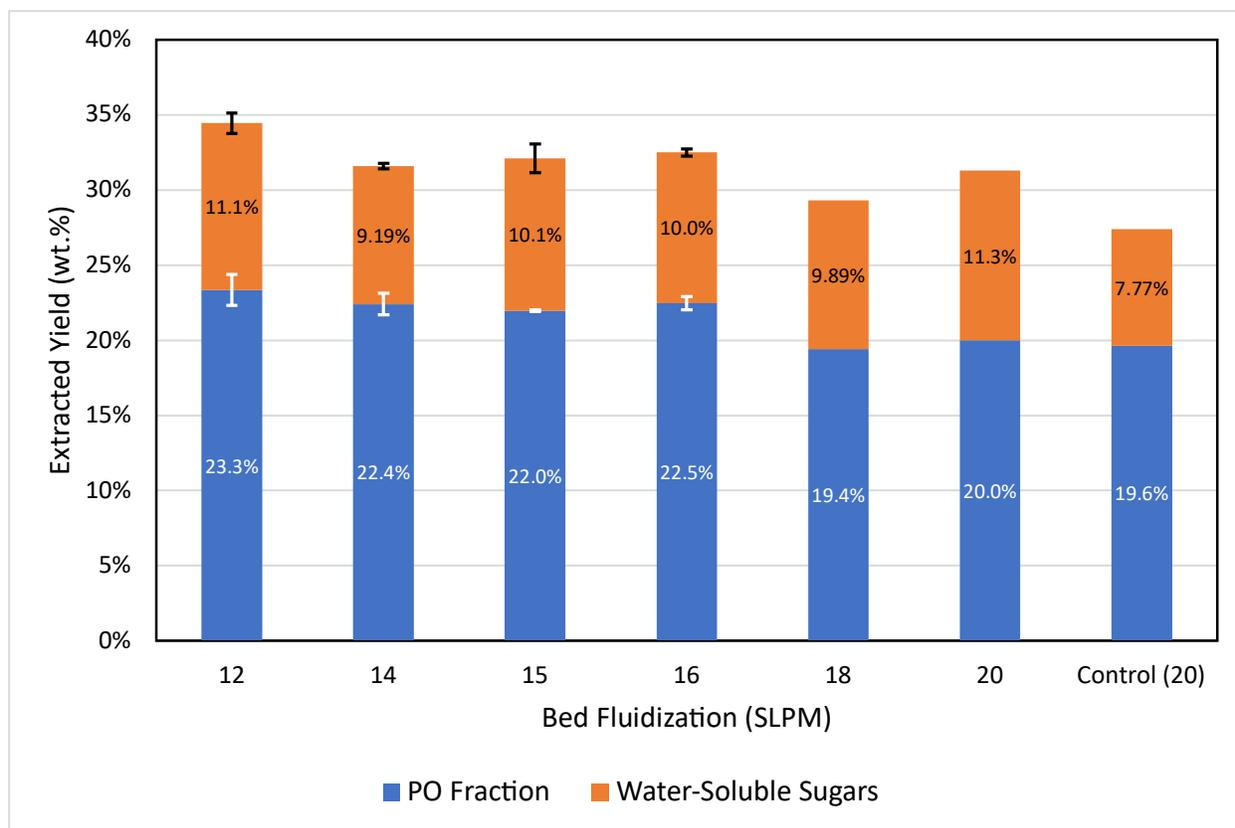
Figure 4.7 Effect of bed fluidization on the extractable yield of phenolic oil and water-soluble sugars
