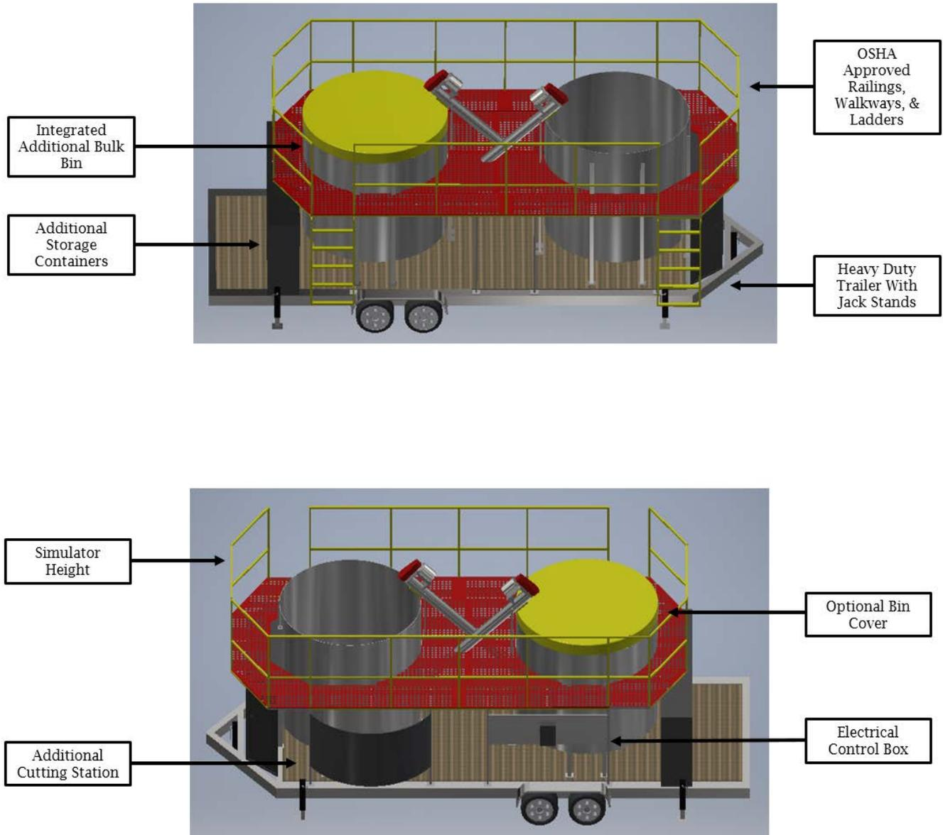
Figure 3-5: Drawing of trailer including basic deminsions
