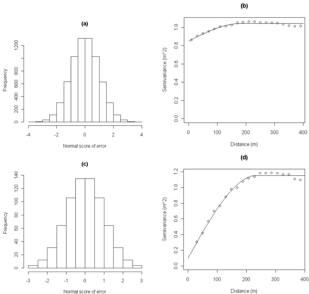
**Figure 4.** Histograms of the normal score-transformed data of (a) 6874 points of DF-DGPS measurement error and (c) 704 points of USGS DEM error with (b and d) their corresponding semivariograms. The solid line on each semivariogram is the semivariogram model.
