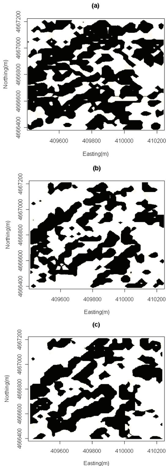
**Figure 9.** Shown in black are the areas that have value greater than  $11.21 \text{ Mg ha}^{-1} \text{ year}^{-1}$  ( $5 \text{ tons acre}^{-1} \text{ year}^{-1}$ ) for erosion rate calculated using simulated DEMs using (a) RTK-DGPS measurements, (b) DF-DGPS measurements, and (c) USGS DEM dataset.
