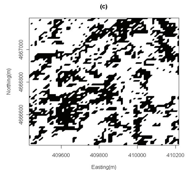
Figure 11. Shown in black are the areas that have erosion rate estimates with CIs containing the  $T$  value of  $11.21 \text{ Mg ha}^{-1} \text{ year}^{-1}$  (5 tons  $\text{acre}^{-1} \text{ year}^{-1}$ ) for DEMs developed using (a) RTK-DGPS measurements, (b) DF-DGPS measurements, and (c) USGS DEM dataset.
