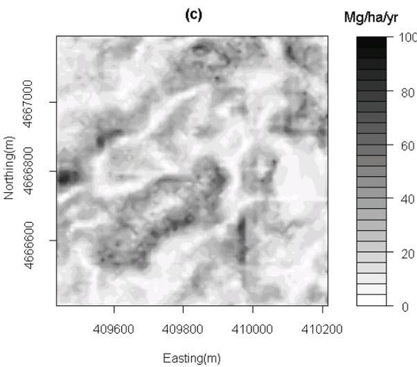
Figure 10. Gray-scale maps of 95% CI of erosion rate estimates calculated using 50 simulated DEMs using (a) RTK-DGPS measurements, (b) DF-DGPS measurements, and (c) USGS DEM dataset.
