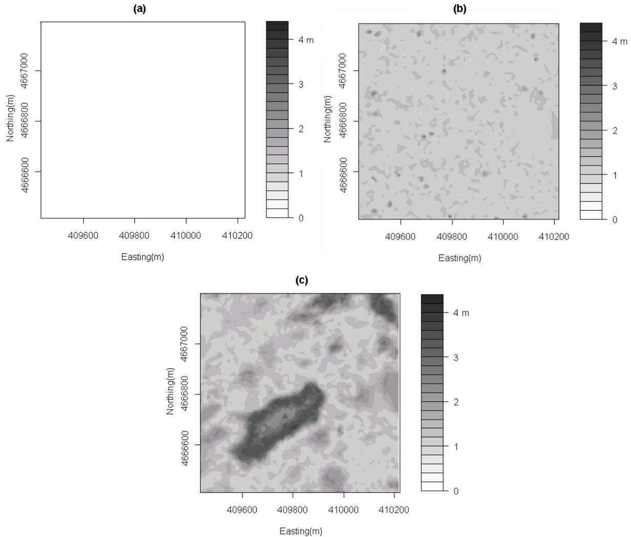
**Figure 7. Gray-scale maps of 95% CI for 50 equiprobable DEMs elevations using (a) RTK-DGPS measurements, (b) DF-DGPS measurements, and (c) USGS DEM dataset.**
