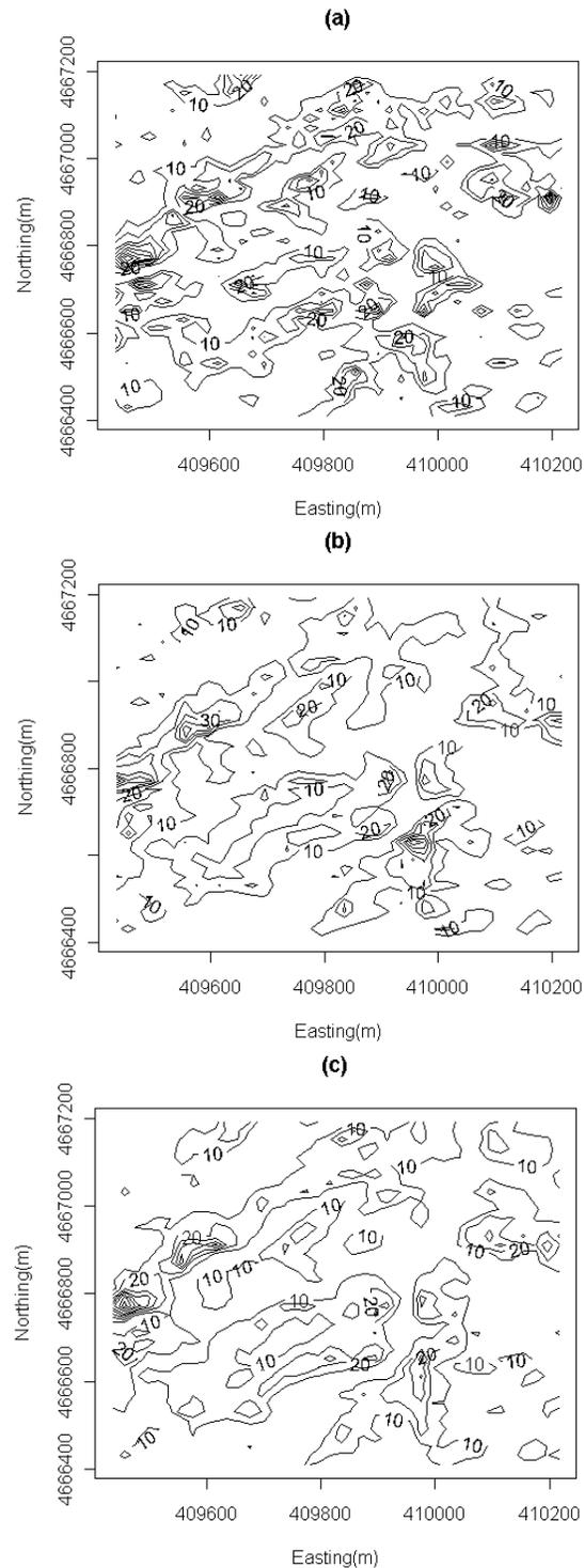
Figure 8. Contour map of erosion rates in  $\text{Mg ha}^{-1} \text{ year}^{-1}$  calculated from kriged DEMs using (a) RTK-DGPS measurements, (b) DF-DGPS measurements, and (c) USGS DEM dataset.
