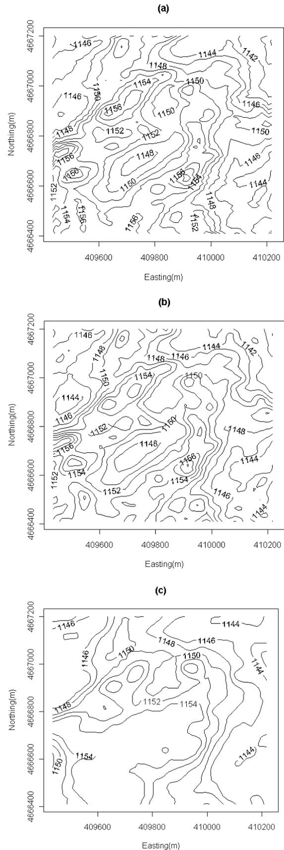
Figure 6. Contour plots of the kriged DEMs developed using (a) RTK-DGPS measurements, (b) DF-DGPS measurements, and (c) USGS DEM dataset.
