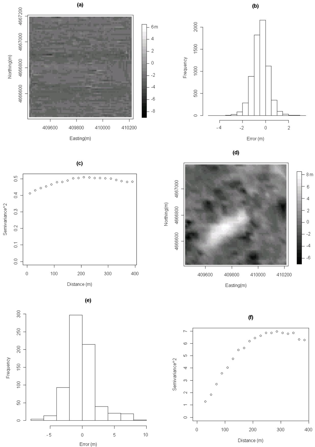
**Figure 3.** Plots and histograms of (a and b) 6874 points of DF-DGPS measurement error and (d and e) 704 points of USGS DEM error with (c and f) their corresponding semivariograms.
