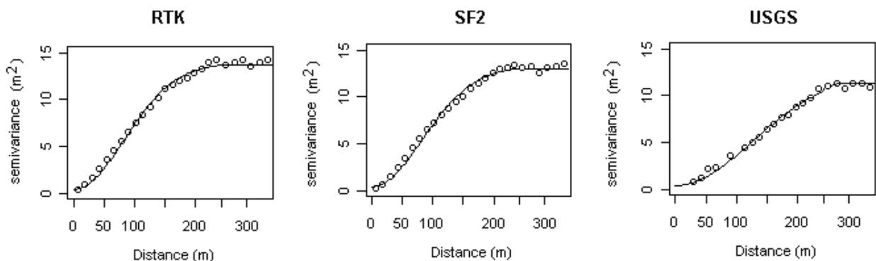
Figure 2. Semivariograms of RTK-DGPS and DF-DGPS measurements and USGS DEM data. The solid line on each semivariogram is the semivariogram model generated using the *gstat* program in R statistical software.
