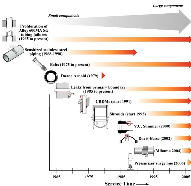
Figure 2. The evolution of passive component failures in NPPs (Staehele, 2010)
