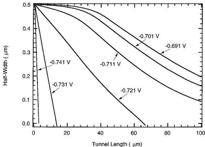
**Figure 4.** Effect of applied potential (parameter on plot) on tunnel shape profiles at  $70^\circ\text{C}$ .
