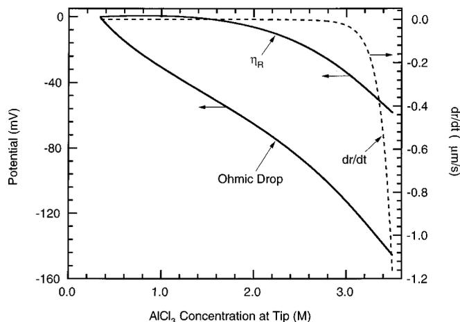
**Figure 3.** Repassivation overpotential  $\eta_R$  and tunnel ohmic potential drop, plotted as a function of the  $\text{AlCl}_3$  electrolyte concentration at the dissolving tunnel tip surface (solid lines). Also shown is the rate of decrease of  $r$ , the half-width of the dissolving surface (dashed line).  $\eta_R$  is found from Eq. 5 and 19, and the ohmic drop is determined by integrating the first term on the right side of Eq. 19.  $dr/dt$  is taken from the exponential term in Eq. 4.
