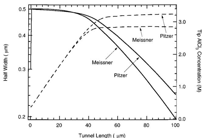
**Figure 6.** Effect of the activity coefficient correlation used on the tunnel shape profile (solid lines) and dissolving tip surface  $\text{AlCl}_3$  concentration (dashed lines) at 70°C. The Meissner correlation is from Ref. 21, and the Pitzer correlation is from Ref. 22, with parameters from Ref. 16.
