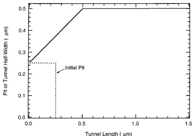
**Figure 1.** Width profiles of tunnels near their entrances. The solid line represents profiles of tunnels formed at 70, 80, and 90°C. The dashed line is the profile of etch pit at the outset of the simulation.
