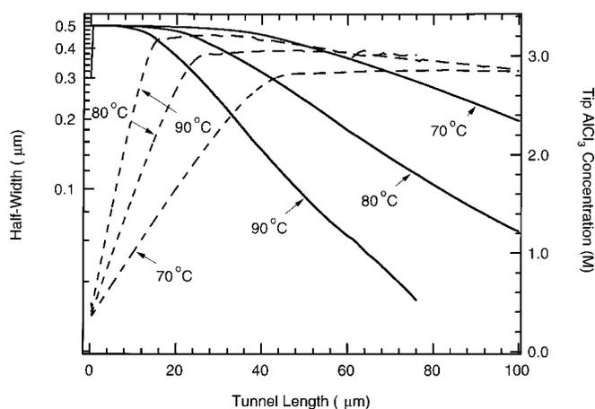
**Figure 2.** Width profiles of tunnels at 70–90°C (solid lines), along with  $\text{AlCl}_3$  electrolyte concentration at the dissolving tunnel tip surface (dashed lines).
