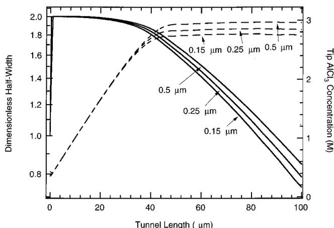
**Figure 5.** Effect of initial pit depth (or half-width) on tunnel shape profiles at 70°C (solid lines). The dimensionless half-width is normalized using the initial pit depth,  $r_0$ . Dashed lines represent the tip electrolyte concentration.
