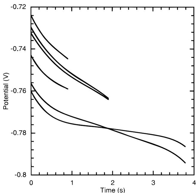
**Figure 4.** Potential transients during current ramps. (a, top) Effect of ramp rate on transients. Parameter is current ramp rate in mA/cm<sup>2</sup>-s. (b, bottom) Several transients for a ramp rate of 20 mA/cm<sup>2</sup>-s. Potentials are corrected using the measured value of the cell ohmic resistance.
