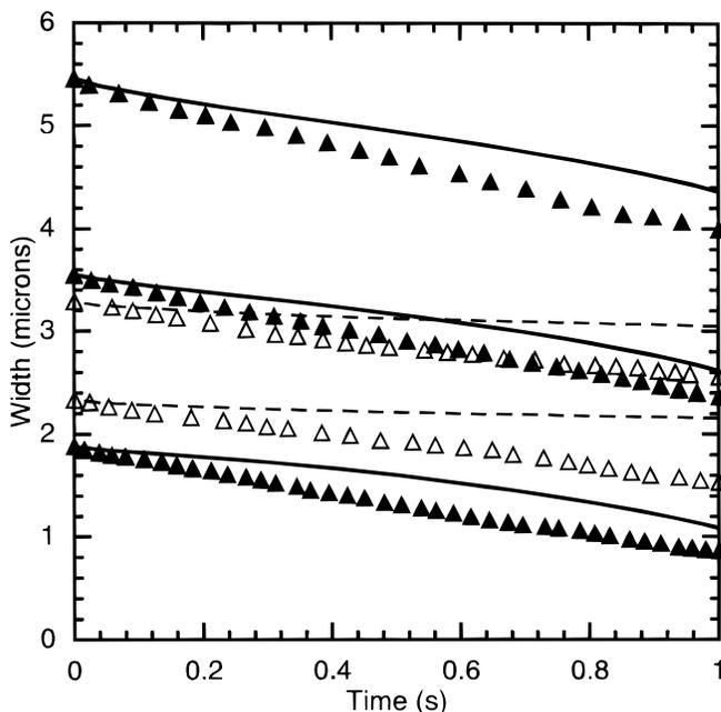
**Figure 8.** Comparison of measured tunnel widths during ramps with predictions by model B. Symbols are width data and lines model calculations. Solid lines and solid symbols represent 20 mA/cm<sup>2</sup>-s experiments and dashed lines and open symbols 10 mA/cm<sup>2</sup>-s experiments.
