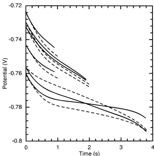
**Figure 7.** Comparison of experimental potential transients (solid lines) with those predicted by model B (dashed lines). (a, top) Potential transients for various current ramp rates. (b, bottom) Several transients at a ramp rate of 10 mA/cm<sup>2</sup>-s. Potentials are corrected using the measured value of the cell ohmic resistance.
