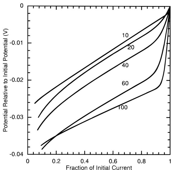
**Figure 6.** Current-potential curves predicted by model A after fitting kinetic parameters and cell resistance to experimental potential transients in Fig. 4a. Potentials are corrected using the measured value of the cell ohmic resistance.
