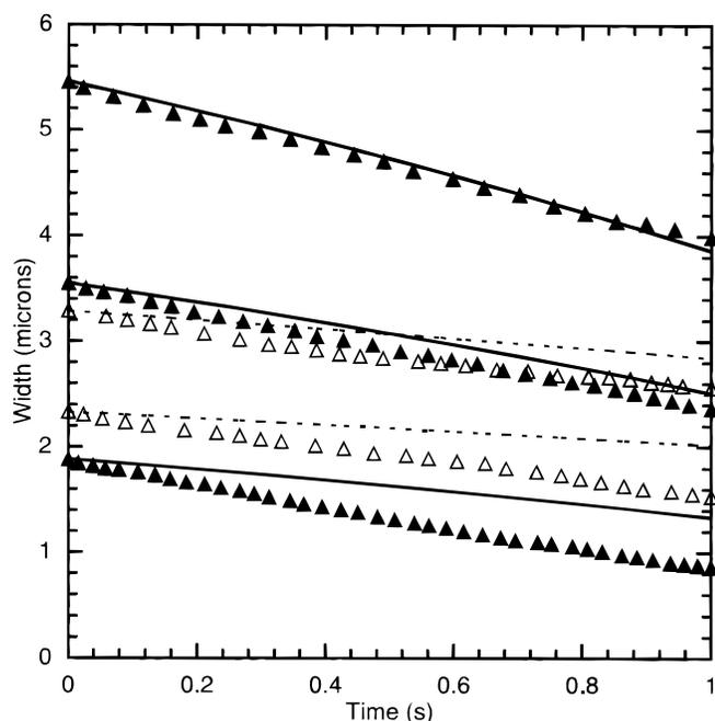
**Figure 3.** Comparison of measured tunnel widths during current ramps with current balance calculations. Symbols are width data and lines calculated values. Solid lines and solid symbols represent 20 mA/cm<sup>2</sup>-s experiments and dashed lines and open symbols 10 mA/cm<sup>2</sup>-s experiments.
