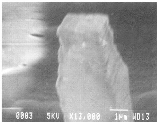
**Figure 1.** Example of an SEM of an oxide replica of an etch tunnel after experiments with a decreasing current ramp. Ramp rate 10  $\text{mA}/\text{cm}^2\text{-s}$ , ramp time 2 s, 5 s at constant current (40  $\text{mA}/\text{cm}^2$ ) before ramp.
