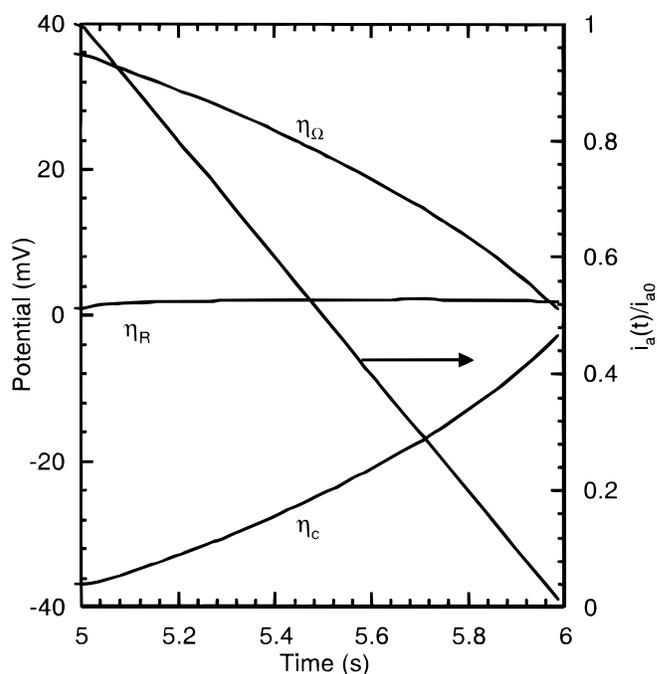
**Figure A-1.** Ohmic and concentration overpotentials in tunnel during current ramp. Ramp rate of 40 mA/cm<sup>2</sup>-s applied after 5 s of etching at constant applied current.
