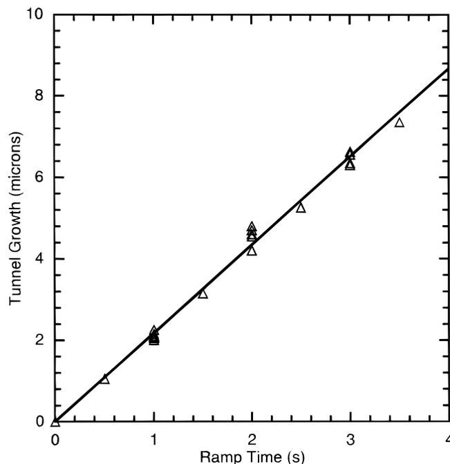
**Figure 2.** Increase of tunnel length during ramp as a function of ramp time. Current ramp rate is 10  $\text{mA}/\text{cm}^2\text{-s}$ . Solid line is a regression fit to the data and has a slope of 2.17  $\mu\text{m}/\text{s}$ .
