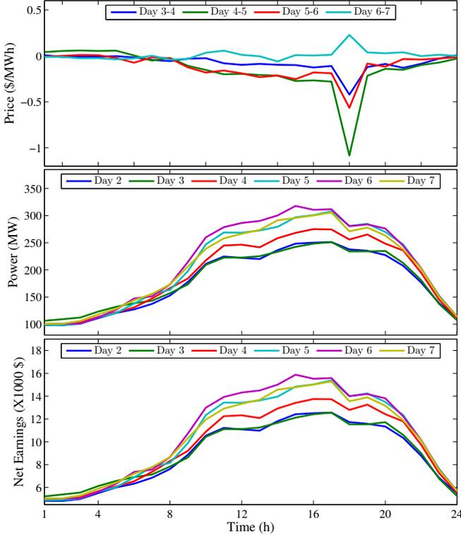
Fig. 6. a) Differences between day-ahead and real-time LMPs; b) The aggregated load profile at bus 4; c) Hourly net earnings of LSE 3 from the two-settlement system.
