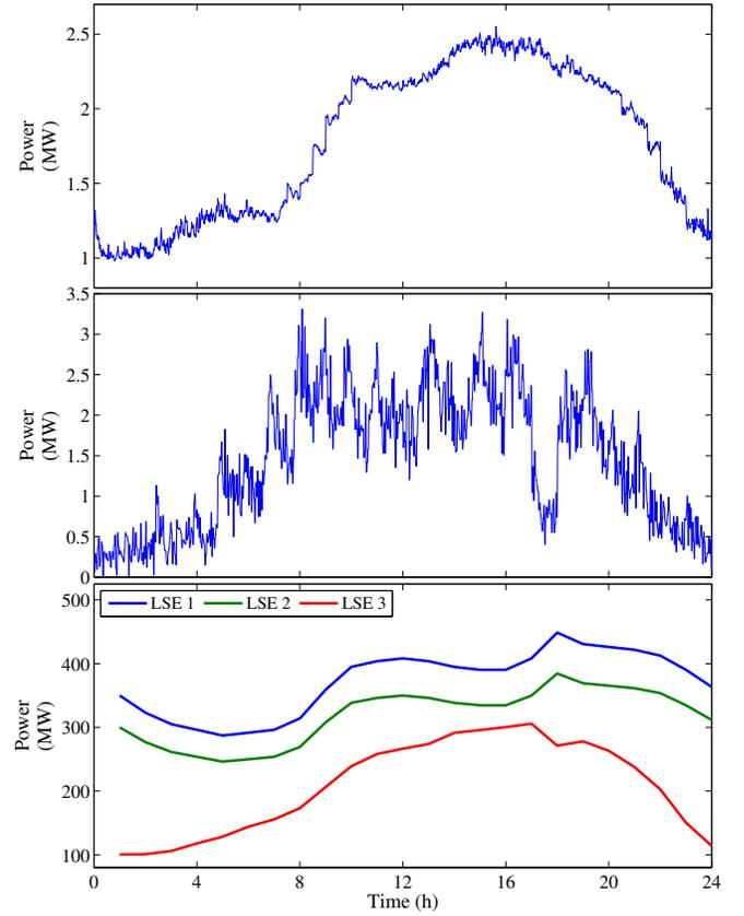
Fig. 2. a) Non-price-responsive load in the distribution feeder; b) Intelligent A/C load in the distribution feeder; c) Daily load profiles for the LSEs, averaged by hour.
