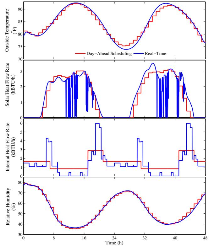
Fig. 3. Variation of environmental parameters for day-ahead scheduling and real-time simulation.
