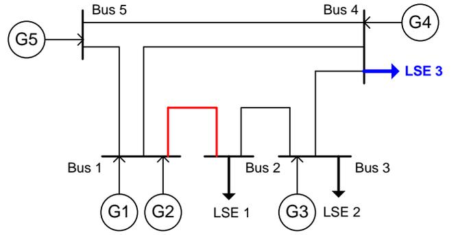
Fig. 1. Power grid for the 5-bus test case.
