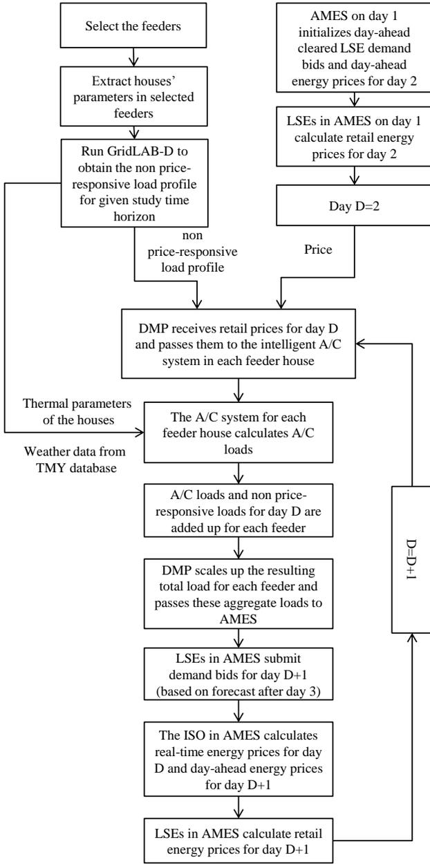
Fig. 5. Flow diagram for a simulation run.
