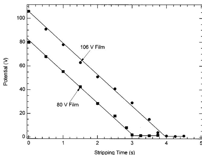
**Figure 5.** Potential at the slope change during reanodizing (see Fig. 4) vs. stripping time in  $\text{H}_3\text{PO}_4$ . Aluminum foils were treated in NaOH for 5 min, and then anodic films were formed to the indicated voltages.
