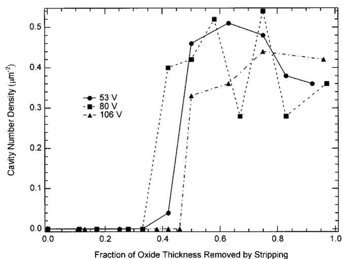
**Figure 9.** Cavity depth distributions in anodic films for foils with 5 min NaOH treatment. Parameter is forming voltage of anodic films.
