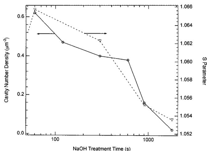
**Figure 12.** Mean void number density in inner portion of anodic films (left axis), plotted vs. NaOH treatment time. Anodizing voltage ranged from 53 to 106 V. Also shown on the right axis is the  $S$  parameter of positron annihilation radiation for NaOH-treated foils without anodic films.
