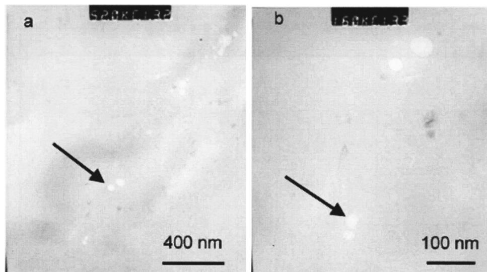
**Figure 2.** TEM images of anodic aluminum oxide film formed to 106 V on aluminum foil treated in NaOH for 5 min. (a) Low magnification and (b) high magnification.
