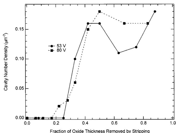
**Figure 11.** Cavity depth distributions in anodic films for foils with 15 min NaOH treatment. Parameter is forming voltage of anodic films.
