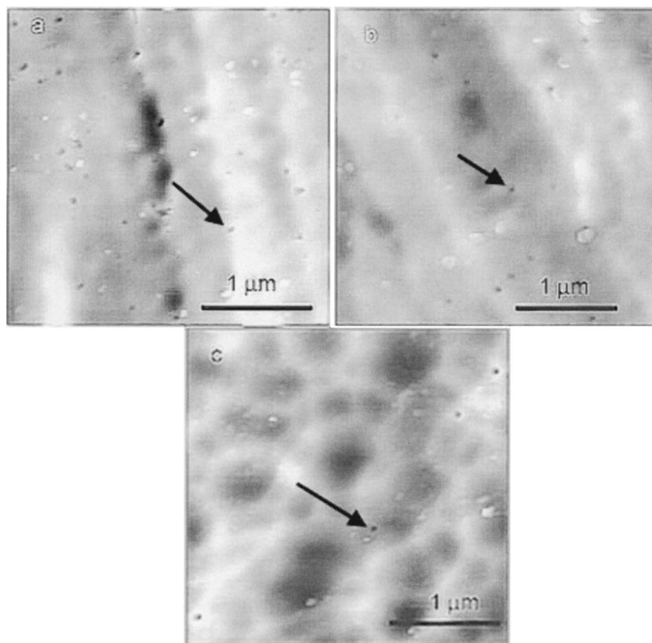
**Figure 10.** AFM images after partial stripping of 80 V anodic films on foils with NaOH treatment times of 1, 2, and 15 min. (a) 1 min NaOH treatment, 90 s stripping (50% of oxide film thickness removed), height contrast 158 nm. (b) 2 min NaOH treatment, 105 s stripping (58% of oxide removed), 158 nm. (c) 15 min NaOH treatment, 90 s stripping (50% of oxide removed), 77 nm.
