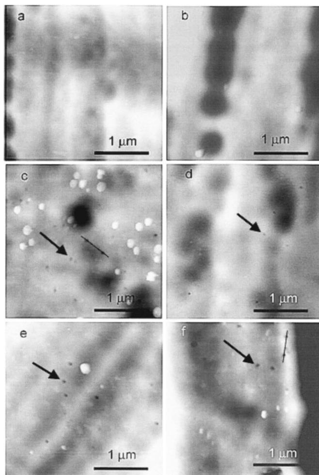
**Figure 6.** AFM images after partial stripping of 106 V anodic films on foils with 5 min NaOH treatment, showing effect of stripping time. Stripping times: (a) 40 s (17% of oxide film thickness removed), height contrast 128 nm; (b) 90 s (38% of oxide removed), 128 nm; (c) 120 s (50% of oxide removed), 116 nm; (d) 150 s (63% of oxide removed), 156 nm; (e) 180 s (75% of oxide removed), 156 nm; (f) 210 s (88% of oxide removed), 147 nm.
