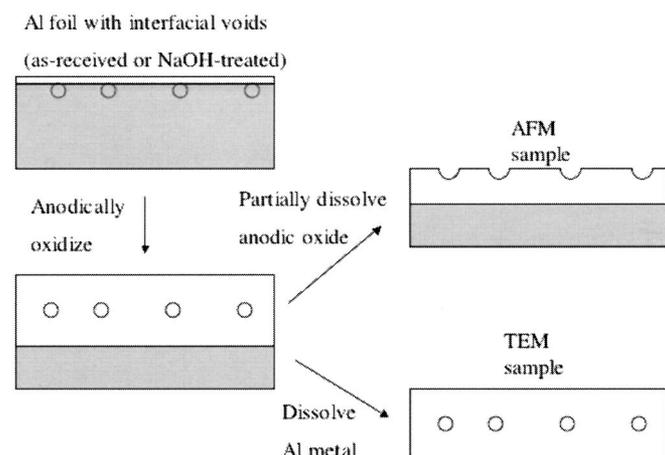
**Figure 1.** Schematic of the experimental protocol leading to preparation of TEM and AFM samples. Voids are represented as circles, and the metal and oxide films by shaded and white areas, respectively. The drawings illustrate the formation of oxide voids by incorporation of pre-existing interfacial voids during anodic film growth; creation of interfacial voids during anodizing and their subsequent incorporation in the film are not depicted.
