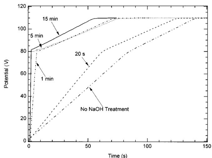
**Figure 4.** Potential-time curves during reanodizing aluminum after partial stripping of the anodic oxide film. Films were originally formed to 106 V and then chemically stripped for 1 min in  $\text{H}_3\text{PO}_4$ . The parameter is the NaOH treatment time prior to the first anodization.
