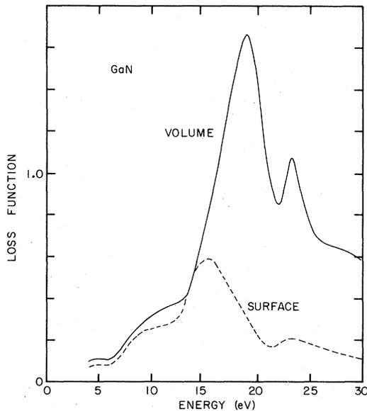
FIG. 3. Volume (solid) and surface (dashed) electron energy loss spectra of Fig. 1 by Kramers-Kronig analysis. These are  $\text{Im}(-1/\tilde{\epsilon})$  and  $\text{Im}[-1/(\tilde{\epsilon})]$ , respectively, for  $q \rightarrow 0$  and  $\vec{E} \perp c$ .
