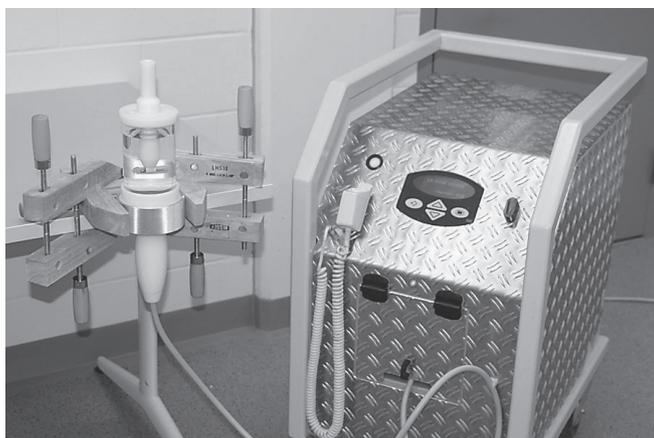
**Figure 1.** Shock wave generator (right) connected to a 35-mm treatment probe shown entering the bottom of a treatment chamber (upper left). The treatment chamber is secured to a table with wooden clamps.
