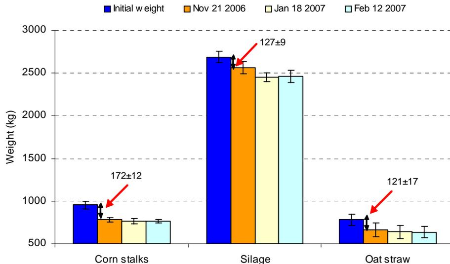
Figure 3. Test unit weight changes during composting process
