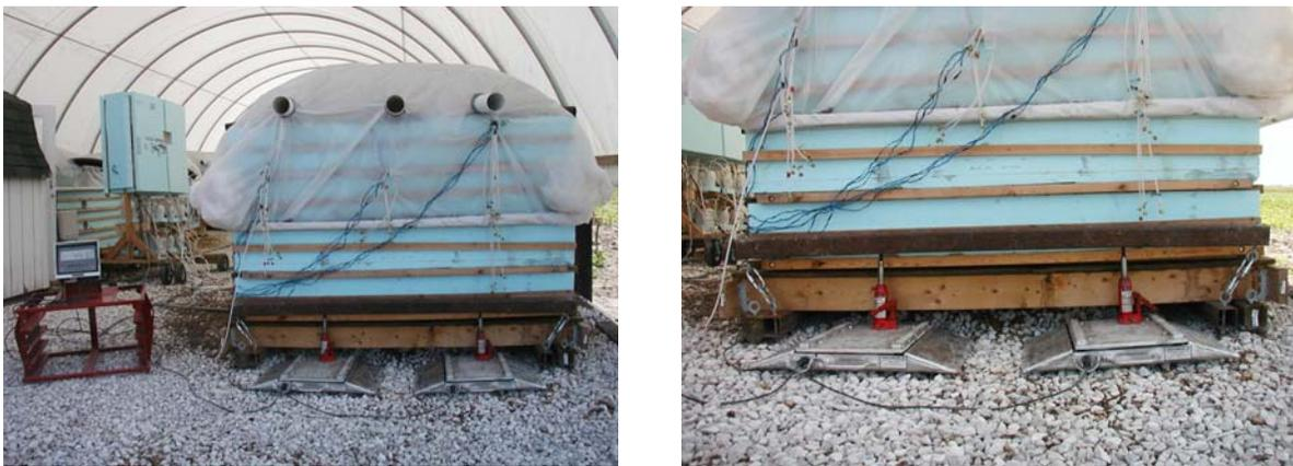
Figure 2. Test platform weight measurement.
