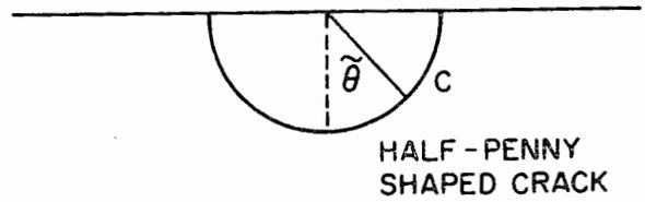
Fig. 7. Schematic of half-penny shaped crack geometry.
