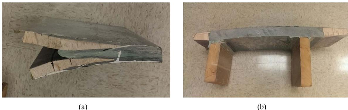
Figure 2. Examples of parts of a WTB showing (a) the sandwich structure leading up to the trailing edge and (b) the complete GFRP spar cap connected to wooden shear webs, which are 5 cm thick.
