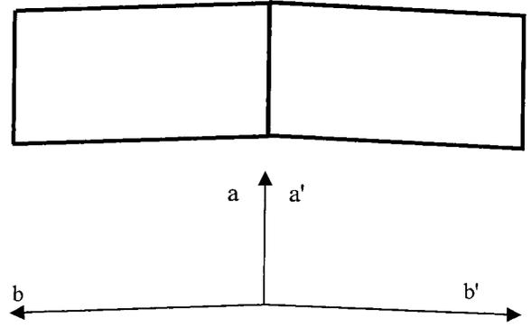
FIG. 3. Scheme for the twin law found in  $\beta$ - $\text{Gd}_5\text{Si}_2\text{Ge}_2$ . The twin axis is the [100] crystallographic axis with  $\mathbf{b}' = \mathbf{b} + \mathbf{a}(2b \cos \gamma)/a$  where  $(2b \cos \gamma)/a = -0.2229$ ,  $a = 7.5891(17) \text{ \AA}$ ,  $b = 14.827 \text{ \AA}$ ,  $c = 7.7862 \text{ \AA}$ , and  $\gamma = 93.262(4)^\circ$ . Cell parameters are from Ref. 6.
