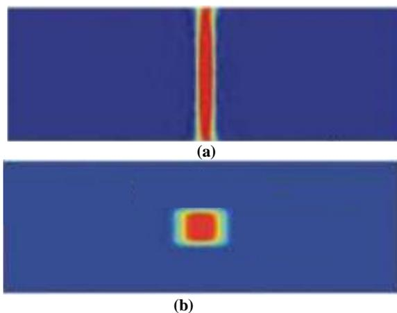
**Fig.2. COMSOL Multiphysics simulations of the core flow pattern at a sheath to core flow rate ratio of 200:10. (a) Core flow pattern at the channel entrance. (b) Core flow pattern after the last chevron.**
