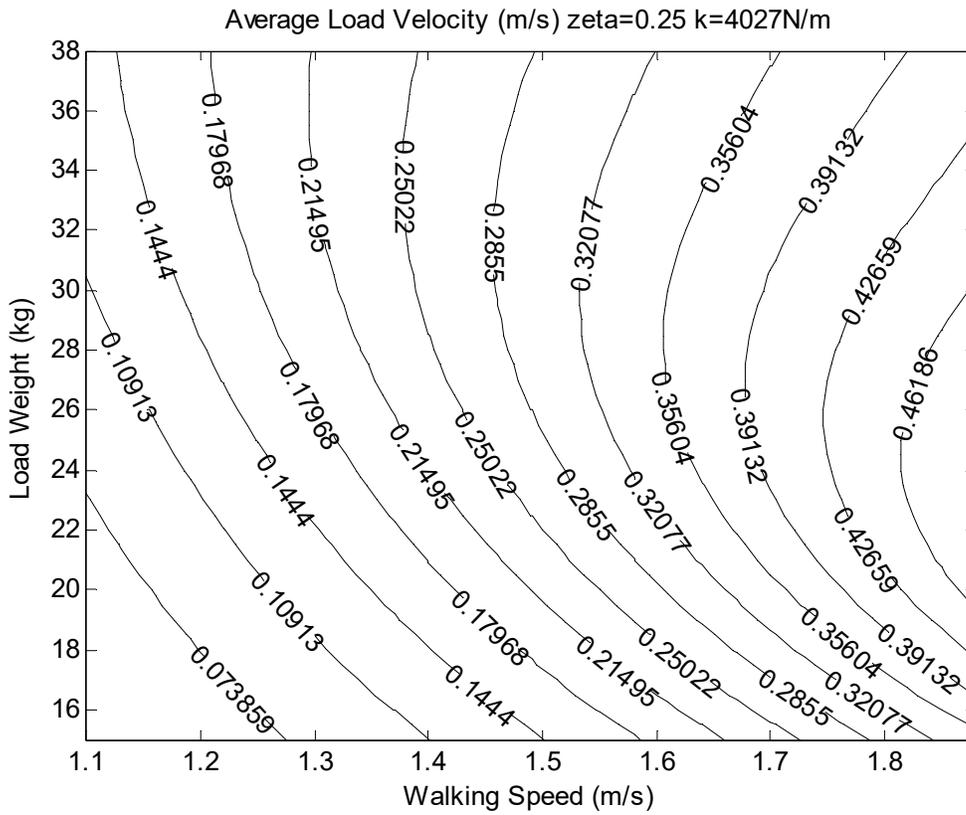
**Figure 11. The predicted  $V_{rms}$  of the suspended load for different walking speed and load mass with a small damping coefficient.**
