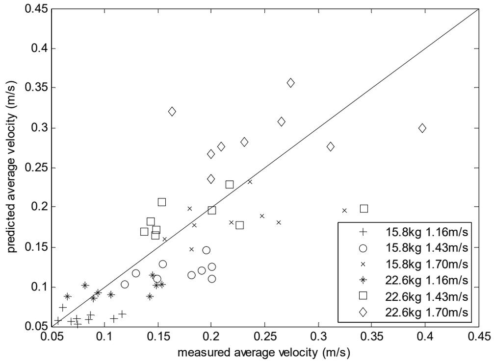
**Figure 9. The scatter plot for the measured vs. predicted RMS of the relative velocity of the suspended load.**
