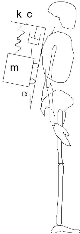
**Figure 7. The configuration of the suspended-load backpack.  $k$ =spring stiffness;  $c$ =damping coefficient;  $m$ =mass.**
