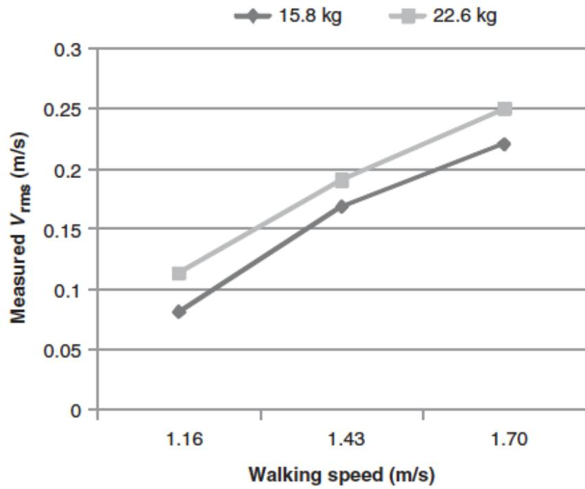
**Figure 10.** The effect of walking speed and load mass on the measured root mean square of the relative velocity of the load to the back pack frame.  $V_{rms}$  is the root mean square of relative velocity between payload and the frame.
