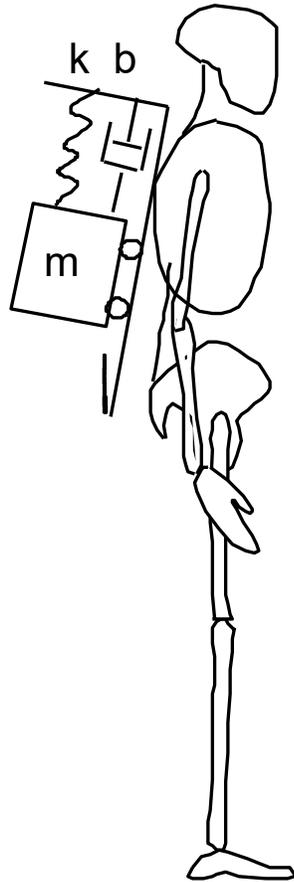
**Figure 1.** The suspended-load backpack.
