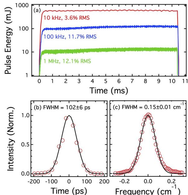
Fig. 3. (a) Burst profiles with 10.5 ms amplifier operation for repetition rates of 10 kHz, 100 kHz, and 1 MHz. (b) Pulse profile measured from autocorrelation with attained FWHM of  $102 \pm 6$  ps. (c) Spectral bandwidth measured using an etalon with FWHM of  $0.15 \pm 0.01$  cm<sup>-1</sup>. The solid lines (b),(c) are Gaussian fits to experimental data (open symbols).
