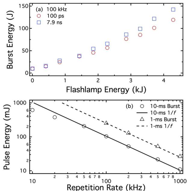
Fig. 2. (a) Total burst energy at 100 kHz as a function of total flashlamp energy for the 100 ps and 7.9 ns oscillators with a burst period of 10 ms. (b) Individual pulse energy at 1064 nm as a function of pulse repetition rate from 10–1000 kHz for a 10 ms burst (100–10,000 pulses) and for 1 ms burst operation from 100–1000 kHz (100–1000 pulses). Measurement uncertainty falls within the symbol size unless indicated.
