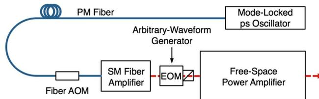
Fig. 1. Schematic of the mode-locked ps oscillator in conjunction with the burst-mode, free-space power amplifier. The acousto-optic modulator is used for pulse-rate reduction via a polarization-maintaining (PM) fiber before amplification in a single-mode (SM) fiber amplifier. A free-space electro-optic modulator (EOM) is used for burst shaping prior to the free-space power amplifier.
