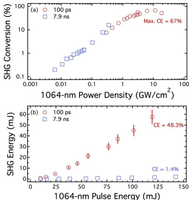
Fig. 4. (a) Second-harmonic conversion efficiency (SHG) in a  $15 \times 15 \times 18$  mm Type-II KD\*P crystal for 100 ps and 7.9 ns pulses as a function of 1064 nm power density. (b) Direct comparison of second-harmonic pulse energy at 100 kHz as a function of fundamental 1064 nm pulse energy for the 100 ps and 7.9 ns pulses under identical laser operating conditions.
