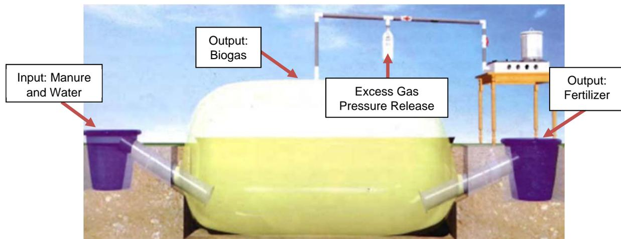
Figure 1: Functional diagram of a plug flow biodigester
