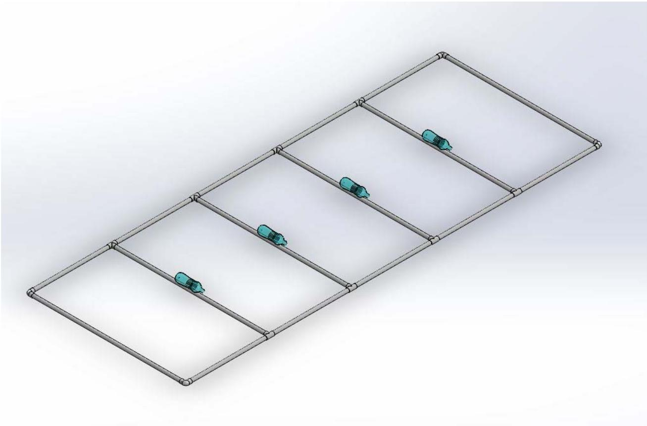
**Figure 3: PVC grid with added water weight**
