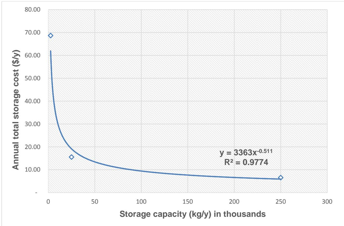
**Figure 6.** Annual total maize storage cost per \$ per kg/y for farm scale maize storage.
