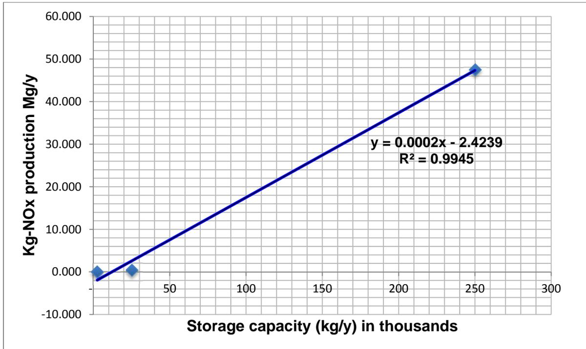
**Figure 8.** NOx emissions for farm scale maize storage.
