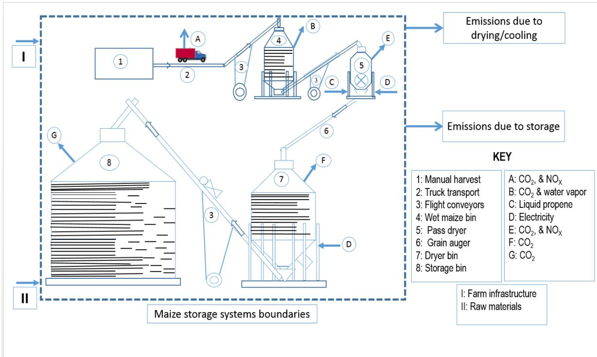
**Figure 3.** Process flow diagram for farm scale maize storage.
