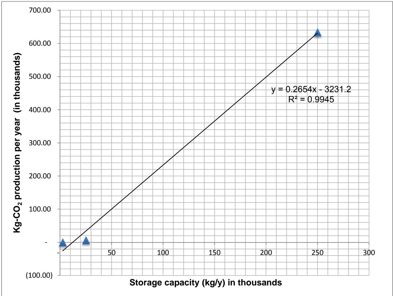
**Figure 7.** CO<sub>2</sub> emissions for farm scale maize storage.
