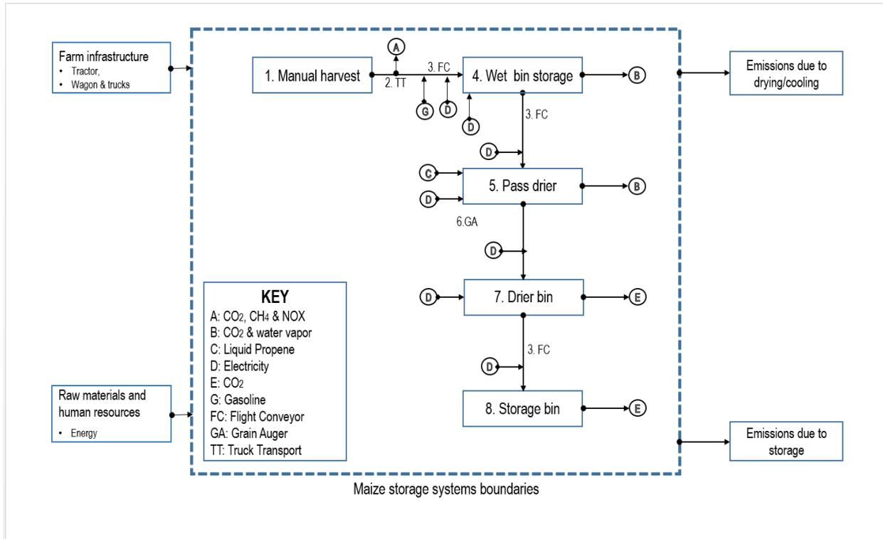
**Figure 4.** Process flow and systems boundaries for farm scale maize storage.
