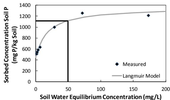
**Figure 2. Example soil phosphorus isotherm demonstrating how the soil phosphorus sorption capacity was determined. Equilibrium soil water P concentration was assumed equal to the flow-weighted average of the applied effluent.**
