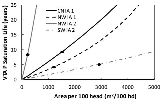
Figure 6. Comparison of VTA phosphorus saturation life expectancies for the top 0.3 m of the soil profile for each of the four sites as a function of VTA area per 100 head. Filled black circles represent the actual VTA area per 100 head at each site.
