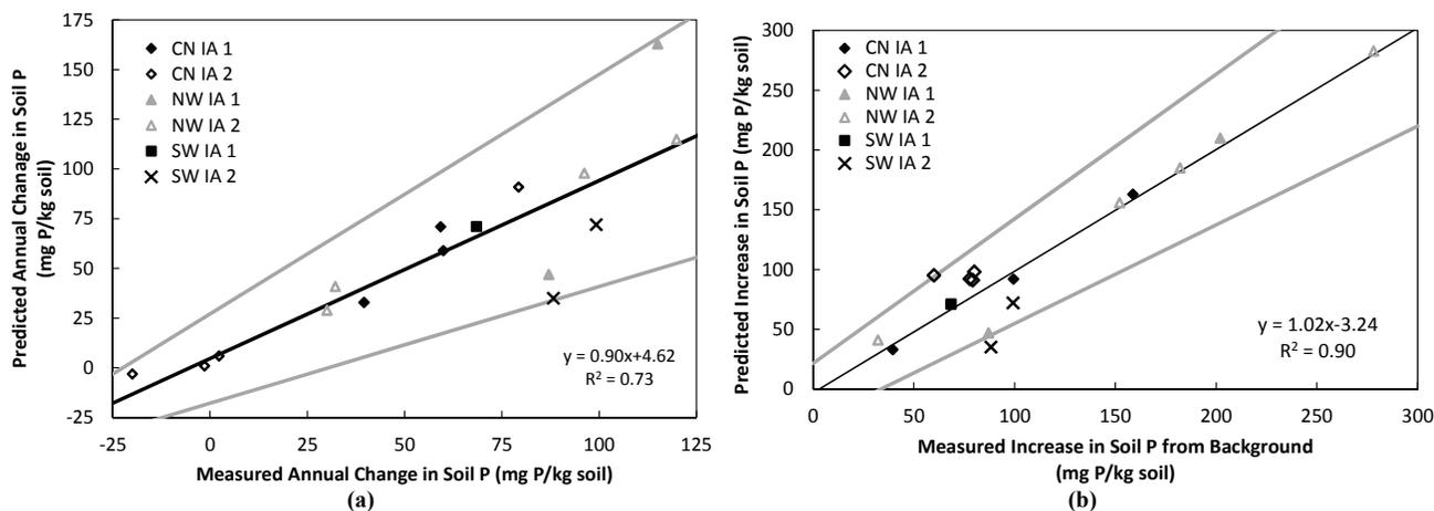
Figure 5. Comparison of soil phosphorus accumulations predicted using the mass balance approach and the monitored phosphorus accumulation shown on (a) annual basis and (b) cumulative basis.
