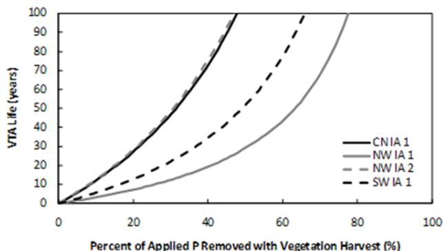
Figure 7. VTA life based on P saturation in the top 0.3 m of the soil profile as a function of the proportion of applied P that needs to be removed with harvested vegetation for four VTAs on feedlots in Iowa.
