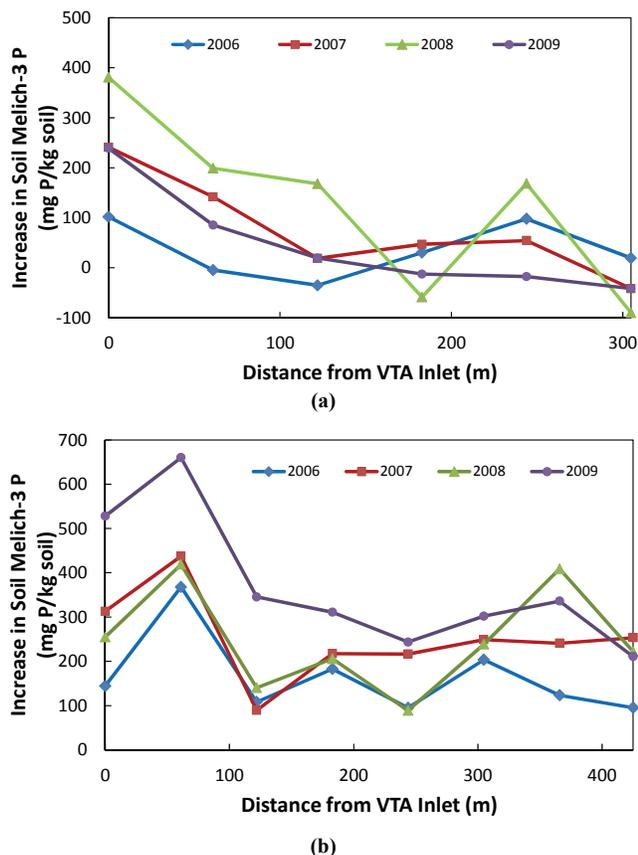
**Figure 3.** Change in surface soil (0 to 0.3 m) Mehlich-3 phosphorus as compared to background concentration as a function of distance from the VTA inlet for (a) Central Iowa 1 and (b) Northwest Iowa 1 vegetative treatment areas.
