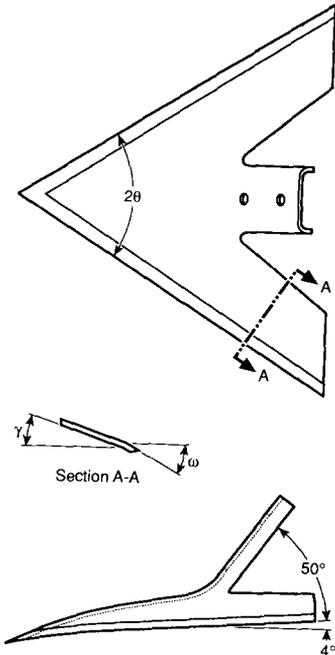
Fig. 1. Sweep geometry with cutting edge inclined to travel direction by angle  $\theta$  and predominant sweep wing rake angle  $\gamma$ .  $\omega$  is edge rake angle. Sweep stem angle used is  $50^\circ$ . Sweep pitch is  $4^\circ$ .
