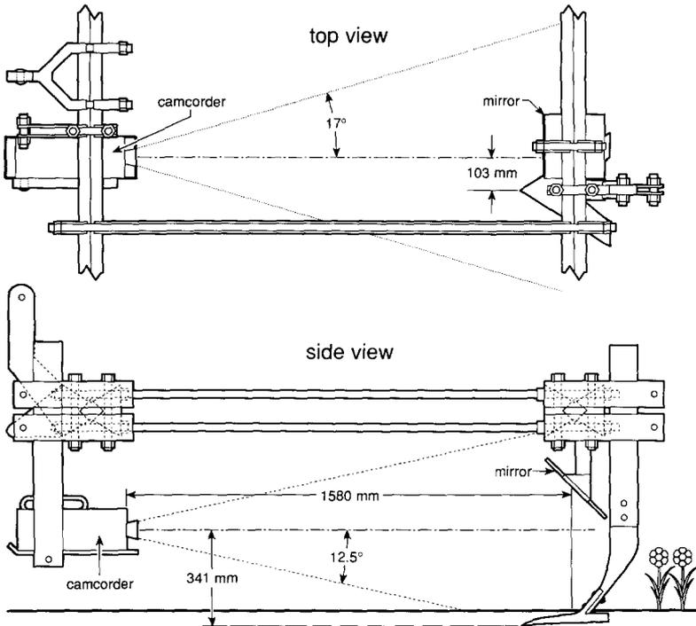
Fig. 4. Toolbar assembly showing location of video camcorder with respect to sweep and overhead mirror. Also shown is video camcorder field of view.
