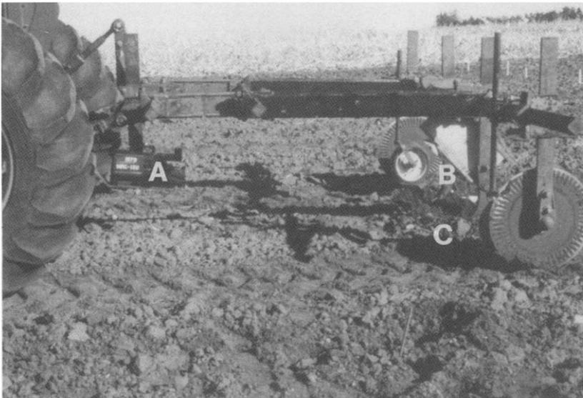
Fig. 3. Toolbar assembly. A, video camcorder; B, mirror; C, sweep.
