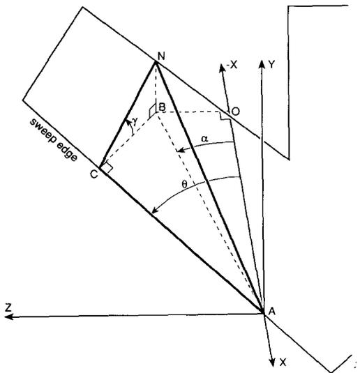
Fig. 2. Soil aggregate flow path,  $AN$ , on the sweep plane.
