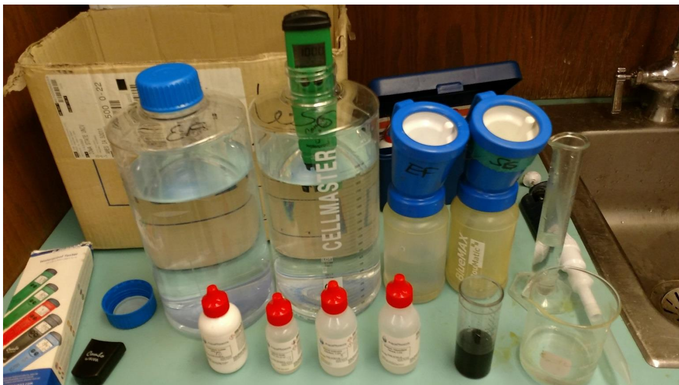
Figure 1. pH /ORP meter and chlorine titration reagents and kit for measuring pH, ORP, and chlorine concentrations over time in EfferCept R , EfferCeptSG R , and water. Initial solutions were made in the 2 liter hard plastic bottles, then transferred to non-siphoning teat dip cups to mimic farm dipper conditions. EF new and EFSG new were stored in plastic 2 liter bottles.
