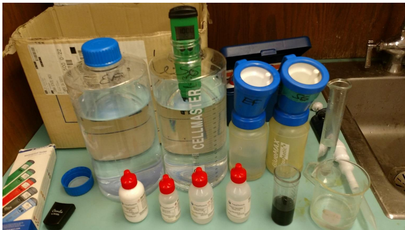
Figure 1. pH /ORP meter and chlorine titration reagents and kit for measuring pH, ORP, and chlorine concentrations over time in EfferCept ® , EfferCeptSG ® , and water. Initial solutions were made in the 2 liter hard plastic bottles, then transferred to non-siphoning teat dip cups to mimic farm dipper conditions. EF new and EFSG new were stored in plastic 2 liter bottles.
