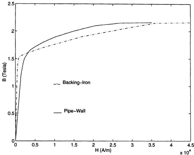
Figure 2. BH curves used in the FEM code.
