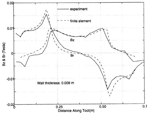
Figure 4. Comparisons of experimental and FEM results with the magnetizer placed in a pipe.
