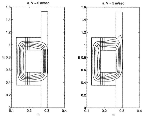
Figure 7. The effect of velocity on the flux lines.
