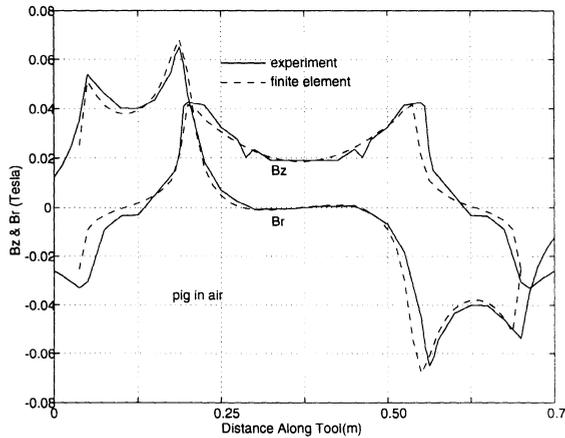
Figure 3. Comparison of experimental and FEM results with the magnetizer placed in air.
