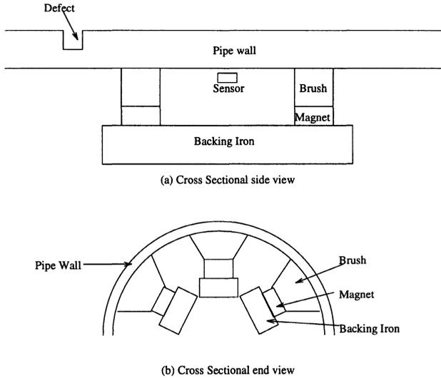
Figure 1. Typical MFL inspection vehicle.
