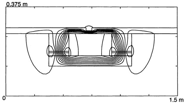
Figure 5. Geometry and field lines corresponding to the MVP formulation (static case).
