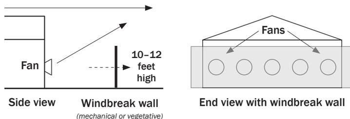
**Figure 2.** Example layout of a windbreak wall for a typical tunnel ventilated building. Windbreak walls should be placed at minimum four fan diameters downwind from the fans.
